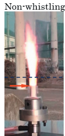
Figure 7 Photograph of the flame of whistle device type B (loading density is below critical density).
