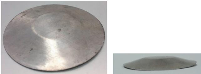
**Figure 2** Final shape of AZ31 plate for case 1.
