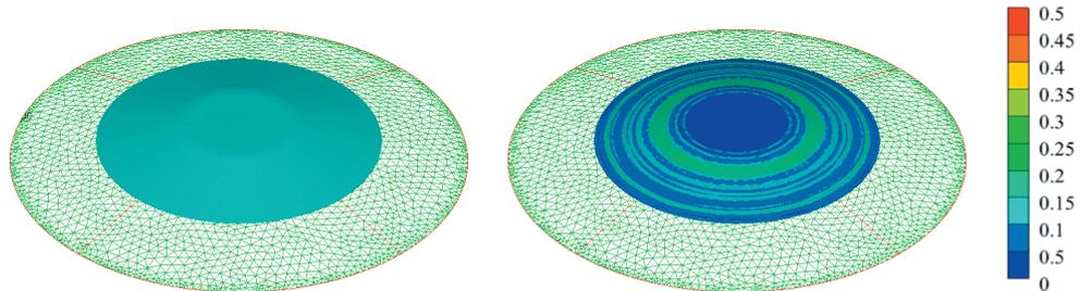
**Figure 5** Final shape of AZ31 plate in case 1. (Left: Material location, Right: Effective plastic strain)
