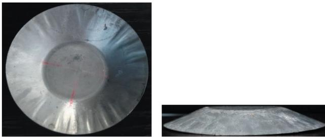
**Figure 3** Final shape of AZ31 plate for case 2.
