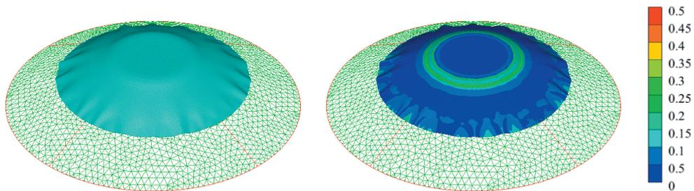
**Figure 6** Final shape of AZ31 plate in case 2. (Left: Material location, Right: Effective plastic strain)
