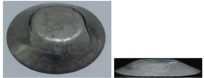
**Figure 4** Final shape of AZ31 plate for case 3.
