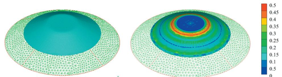
**Figure 7** Final shape of AZ31 plate in case 3. (Left: Material location, Right: Effective plastic strain)
