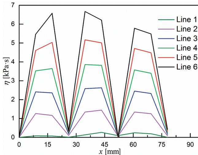
**Figure 4** Viscosity distributions along the lines in XZ section. ( $T = 50\text{ }^{\circ}\text{C}$ ,  $r = 10\text{ r}\cdot\text{min}^{-1}$ ,  $c = 1.20\text{ mL}\cdot\text{g}^{-1}$ )
