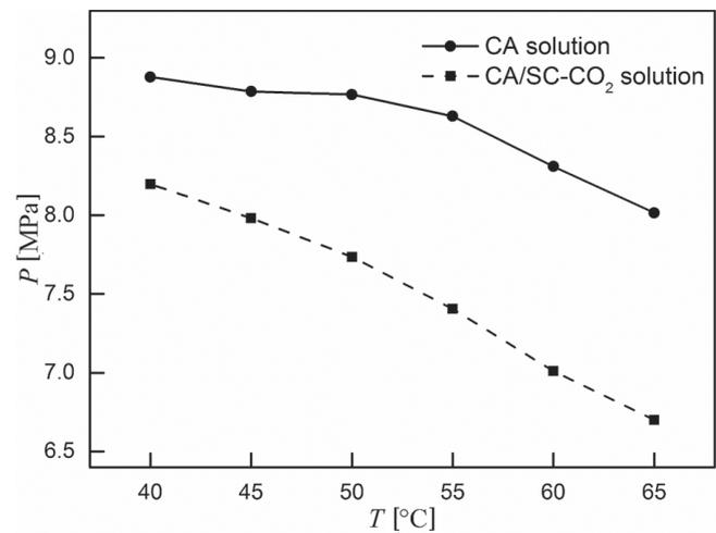
**Figure 9** The average pressure at various temperatures. ( $r = 10\text{ r}\cdot\text{min}^{-1}$ ,  $c = 1.20\text{ mL}\cdot\text{g}^{-1}$ )
