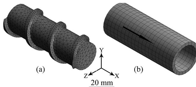
Figure 1 Finite element model of (a) single screw and (b) flow channel.
