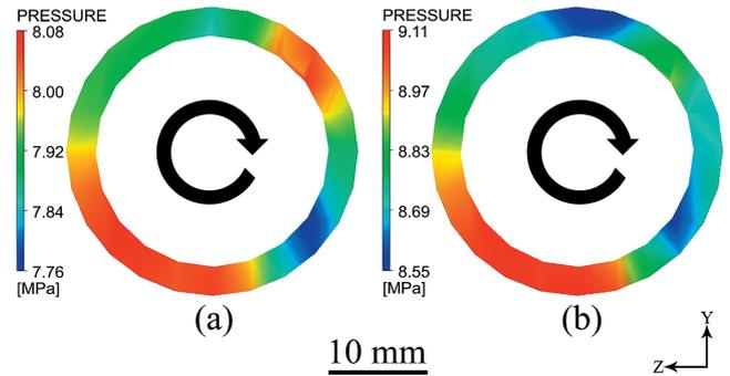
**Figure 5** Pressure distributions in YZ section: (a) CA/SC-CO<sub>2</sub> solution, (b) CA solution. ( $T = 45\text{ }^{\circ}\text{C}$ ,  $r = 10\text{ r}\cdot\text{min}^{-1}$ ,  $c = 1.20\text{ mL}\cdot\text{g}^{-1}$ )
