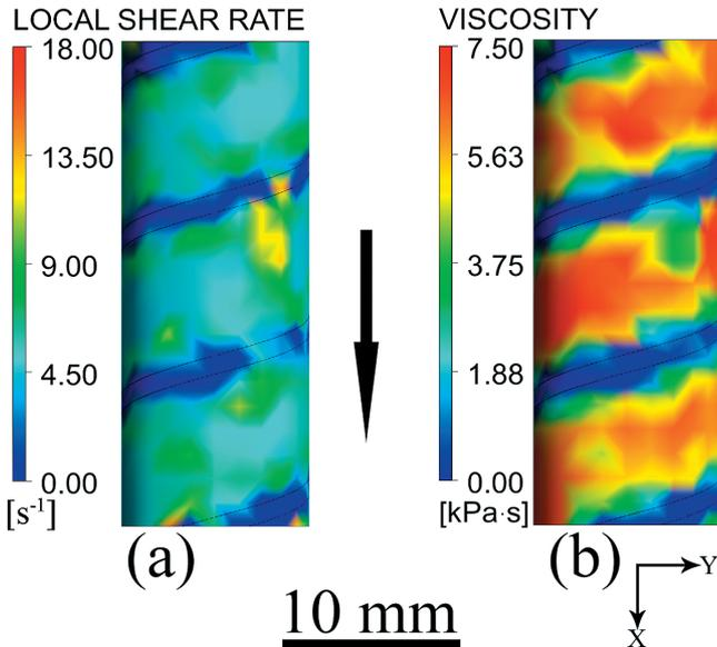
**Figure 3** (a) Shear rate and viscosity (b) distributions in the surface of the fluid. ( $T = 50\text{ }^{\circ}\text{C}$ ,  $r = 10\text{ r}\cdot\text{min}^{-1}$ ,  $c = 1.20\text{ mL}\cdot\text{g}^{-1}$ )
