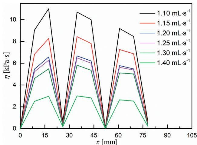
Figure 10 Effects of solvent content on viscosity distributions. ( $T = 50\text{ }^{\circ}\text{C}$ ,  $r = 10\text{ r}\cdot\text{min}^{-1}$ )
