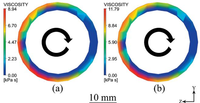
**Figure 6** Viscosity distributions in YZ section: (a) CA/SC-CO<sub>2</sub> solution, (b) CA solution. ( $T = 45\text{ }^{\circ}\text{C}$ ,  $r = 10\text{ r}\cdot\text{min}^{-1}$ ,  $c = 1.20\text{ mL}\cdot\text{g}^{-1}$ )
