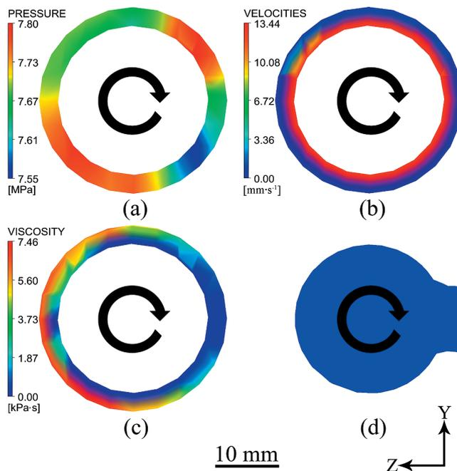
Figure 2 (a) Pressure, (b) velocity, (c) viscosity, and (d) screw distributions in YZ section. ( $T = 50\text{ }^{\circ}\text{C}$ ,  $r = 10\text{ rmin}^{-1}$ ,  $c = 1.20\text{ mL}\cdot\text{g}^{-1}$ )
