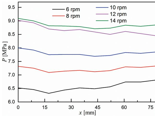
**Figure 7** Effects of screw speed on pressure distributions. ( $T = 50\text{ }^{\circ}\text{C}$ ,  $c = 1.20\text{ mL}\cdot\text{g}^{-1}$ )
