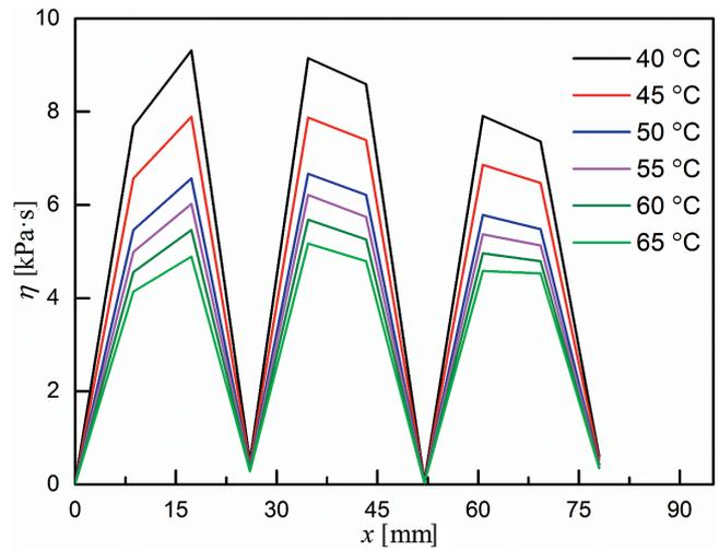
**Figure 8** Effects of temperature on viscosity distributions. ( $r = 10\text{ r}\cdot\text{min}^{-1}$ ,  $c = 1.20\text{ mL}\cdot\text{g}^{-1}$ )
