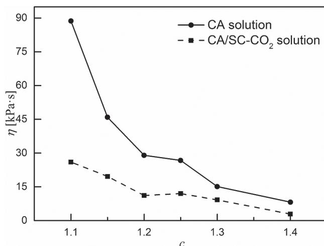
Figure 11 The average viscosity with different solvent content. ( $T = 50\text{ }^{\circ}\text{C}$ ,  $r = 10\text{ r}\cdot\text{min}^{-1}$ )
