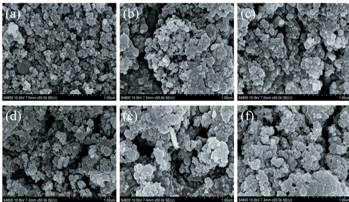
**Figure 3** SEM images of (a)  $(\text{Al}/\text{Fe}_2\text{O}_3)_0$  prepared by ultrasonic and magnetic stirring, (b–f)  $\text{Al}/\text{Fe}_2\text{O}_3/\text{m-DNB}$  (5 wt% NC acts as a binder) composite materials with different m-DNB concentration prepared by a typical electro spray process, (b) 0 wt%, (c) 5 wt%, (d) 10 wt%, (e) 15 wt%, (f) 20 wt%.
