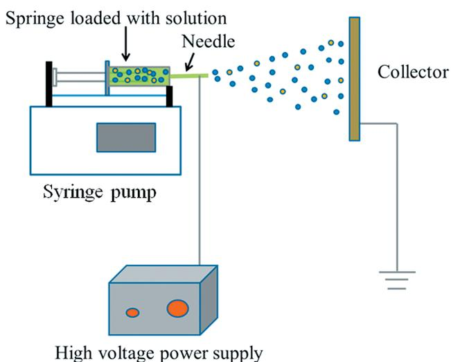
**Figure 1** Schematic diagram of the experimental setup for producing Al/ $\text{Fe}_2\text{O}_3$ /m-DNB composite materials.
