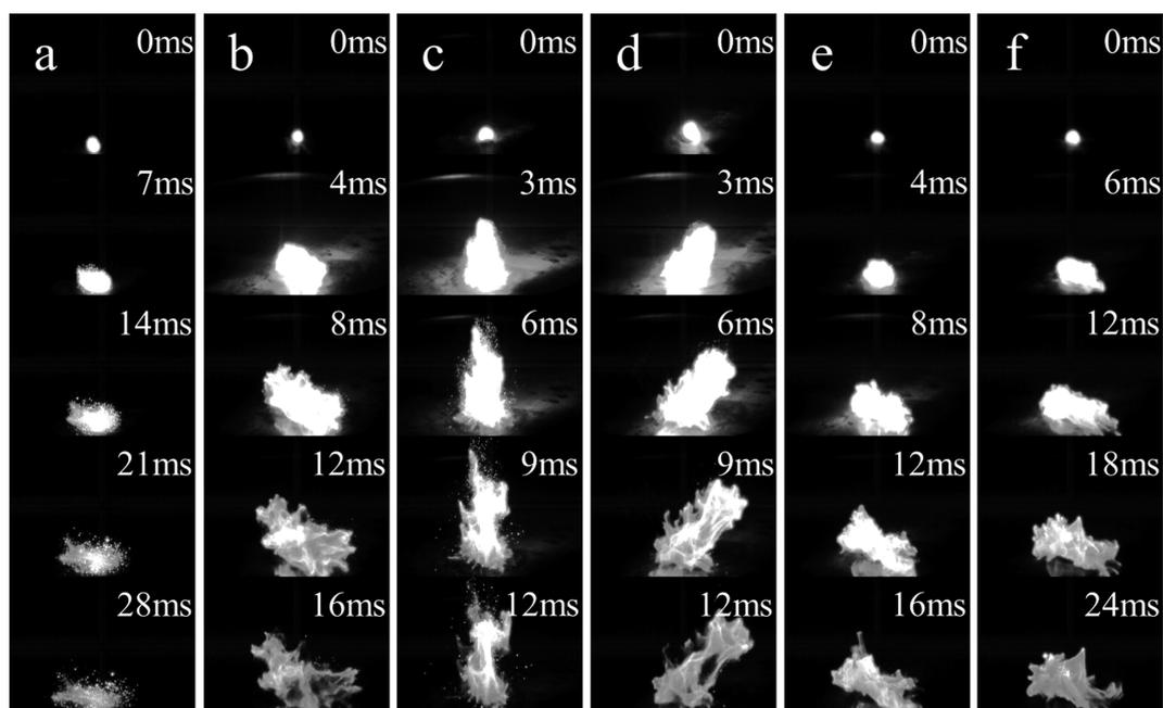
**Figure 6** High speed video images: (a) (Al/Fe<sub>2</sub>O<sub>3</sub>)<sub>0</sub> prepared by ultrasonic and magnetic stirring; (b–f) Al/Fe<sub>2</sub>O<sub>3</sub>/m-DNB (5 wt% NC acts as a binder) with different m-DNB concentration prepared by a typical electro spray process. (b) 0 wt%, (c) 5 wt%, (d) 10 wt%, (e) 15 wt%, (f) 20 wt%.
