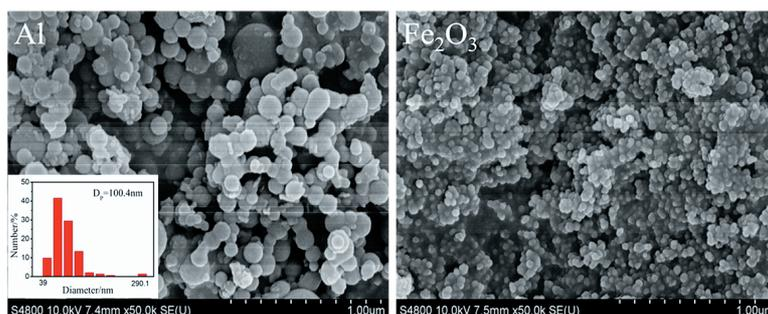
**Figure 2** SEM images of raw Al and raw  $\text{Fe}_2\text{O}_3$  before electro-spray and the size distribution of original Al (where,  $D_p$  is the average diameter of aluminum nanopowders).
