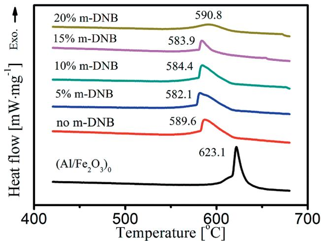
**Figure 5** DSC curves of Al/Fe<sub>2</sub>O<sub>3</sub>/m-DNB (5 wt% NC acts as a binder) composite materials with different m-DNB concentration prepared by a typical electro spray process, and (Al/Fe<sub>2</sub>O<sub>3</sub>)<sub>0</sub> prepared by ultrasonic and magnetic stirring.
