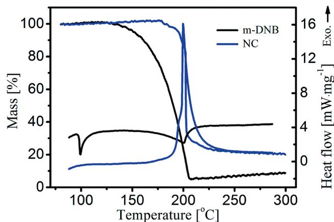
**Figure 4** TG/DSC curves of NC and m-DNB.
