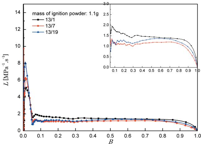
**Figure 5** Dynamic vivacity curves of the three kinds of TEGDN propellant when the mass of ignition powder is 1.1 g (the inset figure shows detail of the curves with the ignition event removed).
