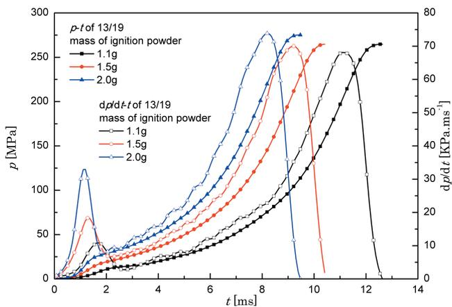
**Figure 8** Pressure-time ( $p-t$ ) curves and  $dp/dt-t$  curves of 13/19 TEGDN propellant at three ignition masses of 1.1 g, 1.5 g and 2.0 g.
