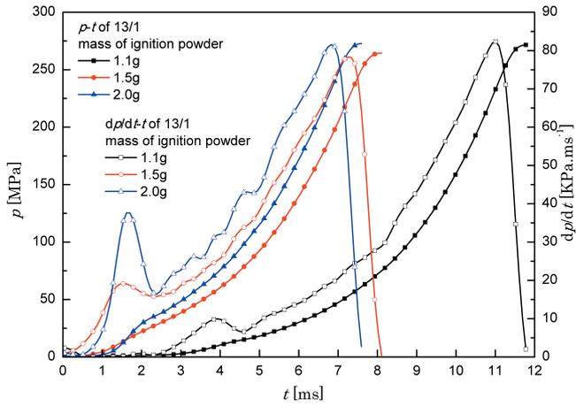
**Figure 6** Pressure-time ( $p-t$ ) curves and  $dp/dt-t$  curves of 13/1 tube TEGDN propellant at three ignition masses of 1.1 g, 1.5 g and 2.0 g.
