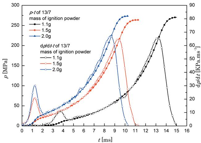
**Figure 7** Pressure-time ( $p-t$ ) curves and  $dp/dt-t$  curves of 13/7 TEGDN propellant at three ignition masses of 1.1 g, 1.5 g and 2.0 g.
