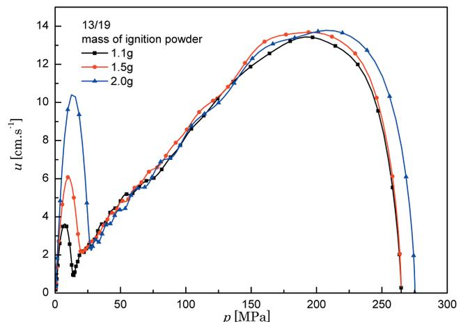
**Figure 11** Burn rate ( $u-p$ ) curves of 13/19 TEGDN propellant at three ignition masses of 1.1 g, 1.5 g and 2.0 g.
