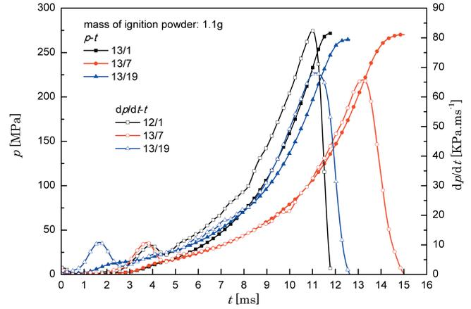
**Figure 3** Pressure-time ( $p-t$ ) curves and  $dp/dt-t$  curves of the three kinds of TEGDN propellant when the mass of ignition powder is 1.1 g.
