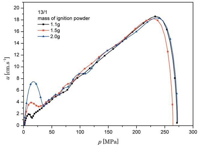
**Figure 9** Burn rate ( $u-p$ ) curves of the 13/1 TEGDN propellant at three ignition masses of 1.1 g, 1.5 g and 2.0 g.
