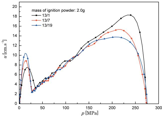
**Figure 13** Burn rate ( $u-p$ ) curves of the three kinds of TEGDN propellant when the mass of ignition powder is 2.0 g.
