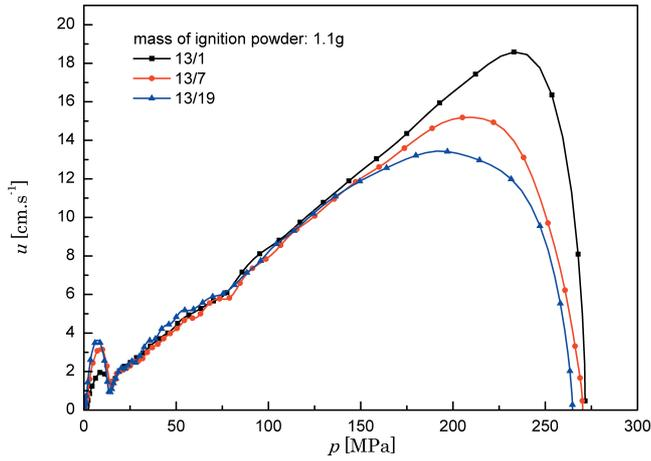
**Figure 4** Burn rate ( $u$ - $p$ ) curves of the three kinds of TEGDN propellant when the mass of ignition powder is 1.1 g.
