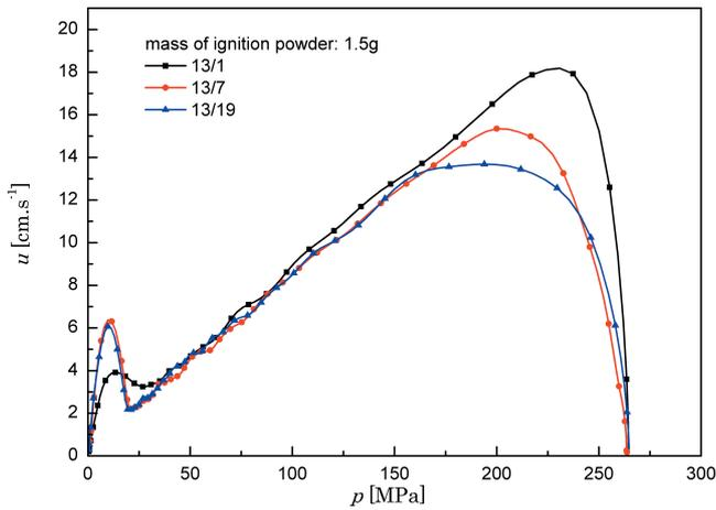
**Figure 12** Burn rate ( $u-p$ ) curves of the three kinds of TEGDN propellant when the mass of ignition powder is 1.5 g.
