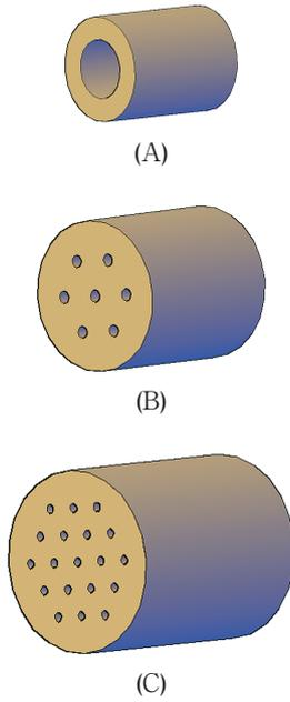
**Figure 1** 3D graph of three kinds of TEGDN propellant grains: (A) 13/1 TEGDN propellant grain; (B) 13/7 TEGDN propellant grain; (C) 13/19 TEGDN propellant grain.
