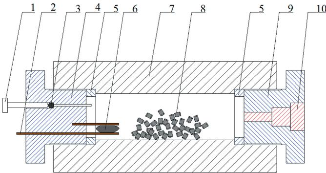
**Figure 2** Schematic of closed bomb test setup: 1- bleed valve, 2 - igniter rod, 3 - steel ball, 4 - ignition bolt, 5 - washer, 6 - ignition powder, 7 - main body, 8 - tested propellant sample, 9 - bolt with pressure transducer, 10 - pressure gauge.
