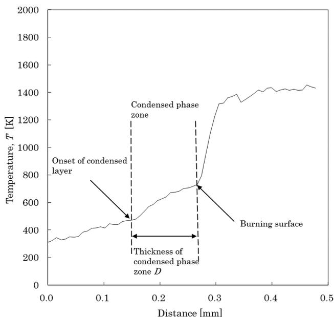
**Figure 2 (b)** Typical temperature history of a burning G15B/AN/CuO mixture pellet.
