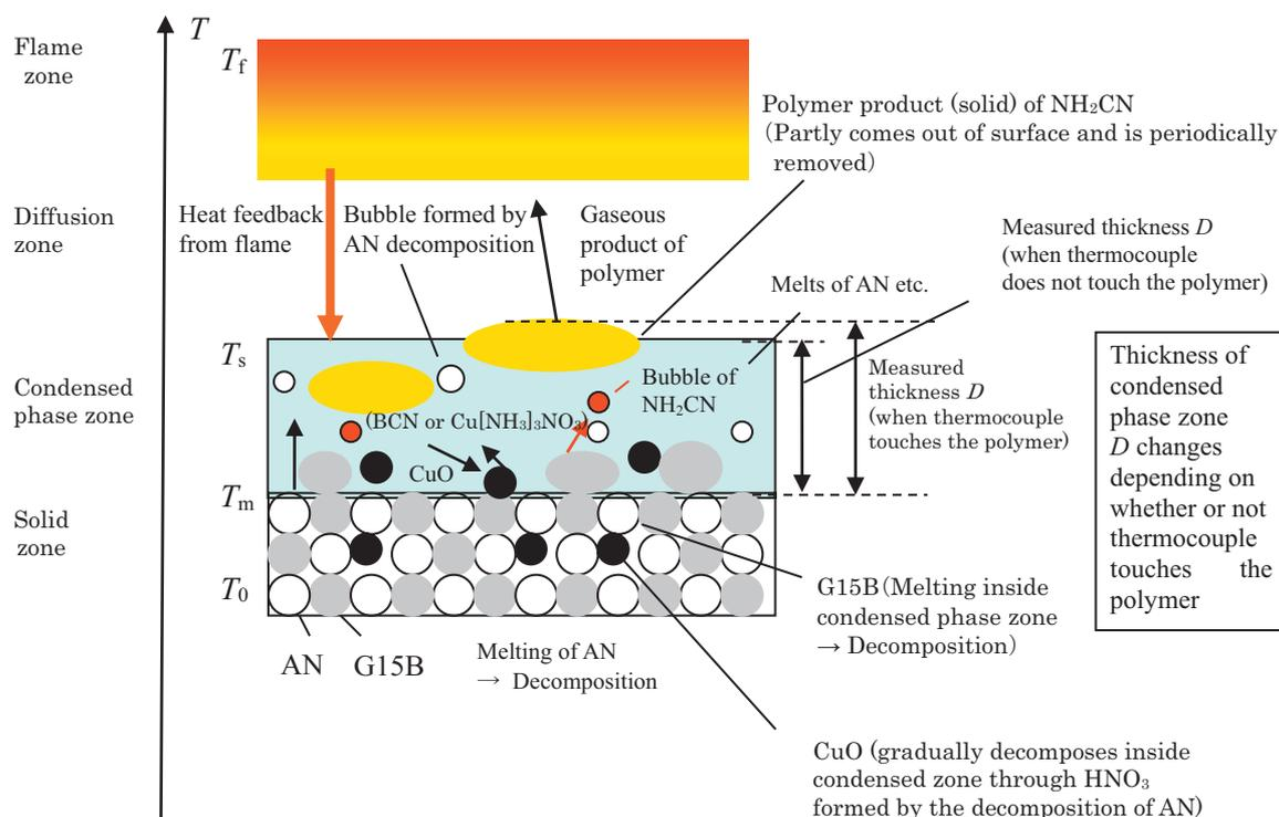
**Figure 3** Estimated burning mechanism of G15B/AN/CuO mixture.
