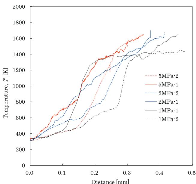
**Figure 2 (a)** Temperature histories of burning G15B/AN/CuO mixture pellets.
