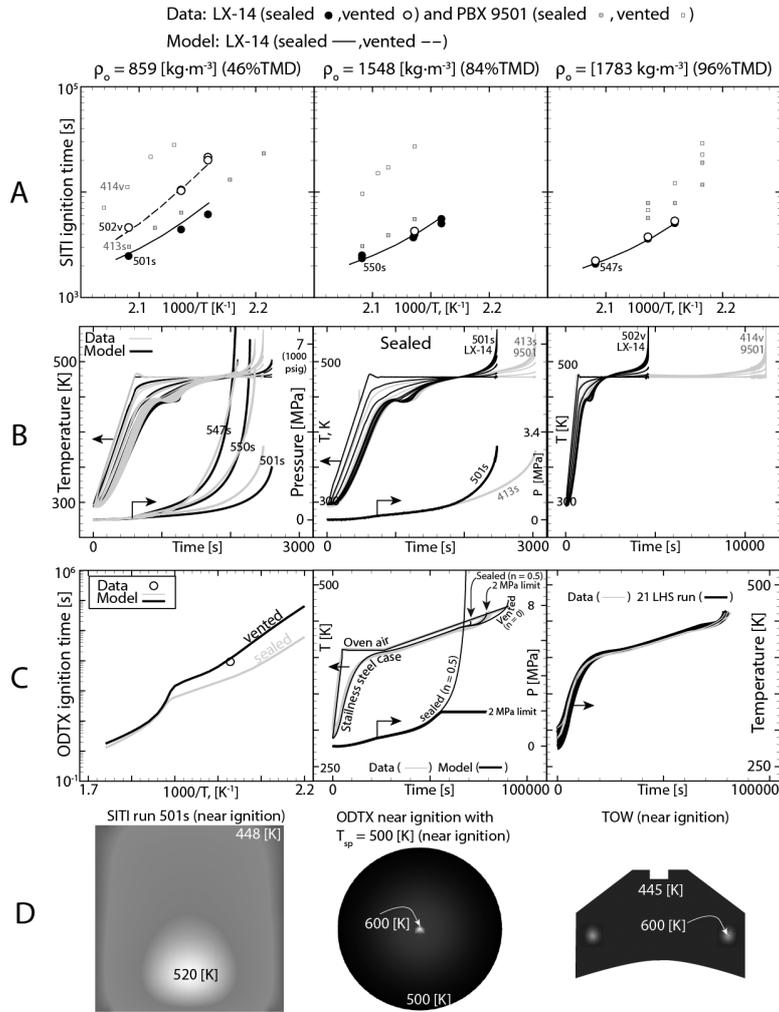
**Figure 3** A) SIT ignition times, B) SIT temperature and pressure profiles, C) ODTX ignition times and TOW temperature and pressures, and D) temperature contours near ignition for SIT, ODTX, and TOW.
