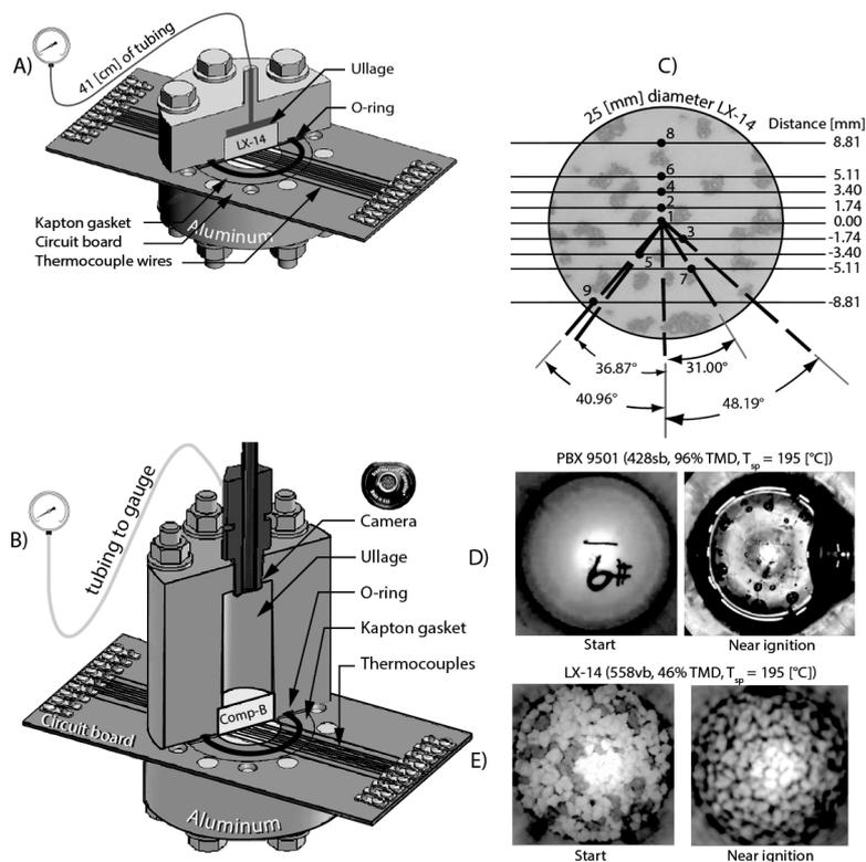
**Figure 1** SITI schematic with A) small expansion gap and B) large head space showing borescope camera. C) Cross-section of LX-14 in the SITI apparatus showing thermocouple locations. Borescope images at the beginning and near ignition for D) PBX 9501 and E) LX-14.
