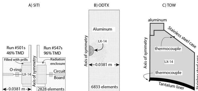
Figure 2 Schematic for A) SITI, B) ODTX, and C) TOW experiments.
