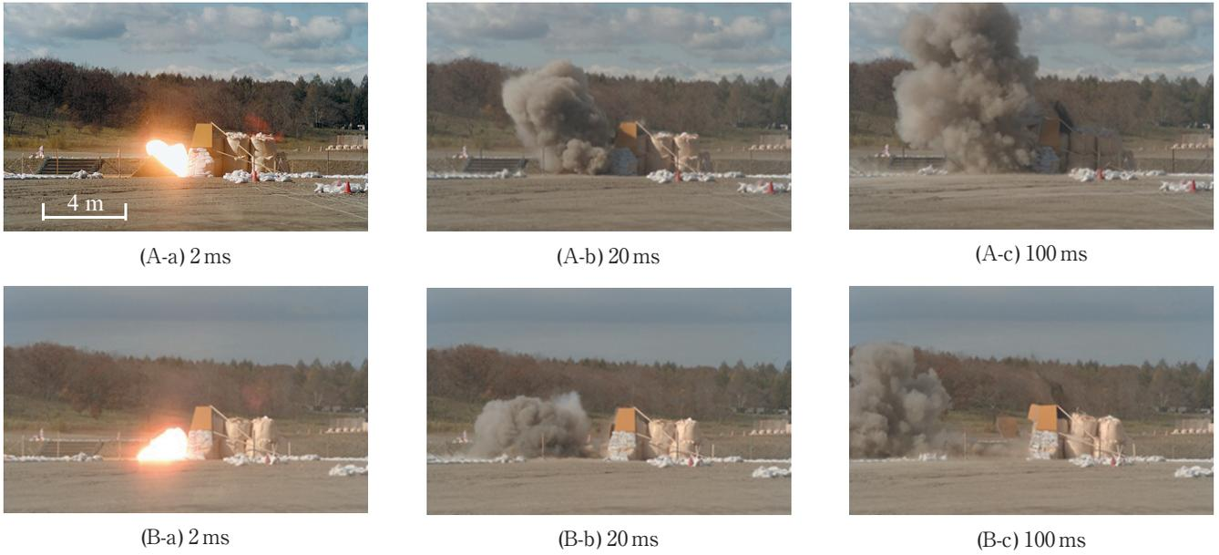
**Figure 2** High-speed photographs captured at (a) 2 ms, (b) 20 ms, and (c) 100 ms after ignition in case of (A) No.1-1 (with the dike) and (B) No.1-2 (without the dike).
