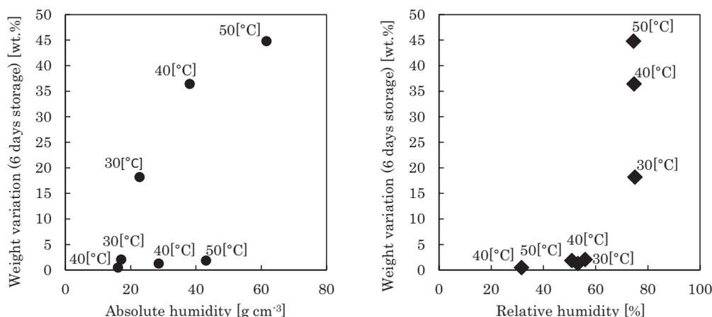
Figure 9 Effect of humidity parameter. (Sample A after 6 days storage)
