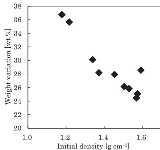
Figure 5 Effect of initial density. (Sample C) [75%RH, 40 °C, 6 days].
