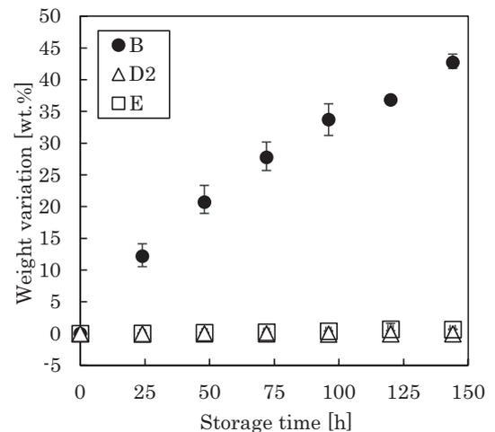
Figure 4 Weight variation by aging test. (Sample B, D, E) [75%RH, 40 °C].
