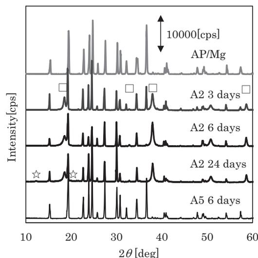
Figure 1 XRD peak of aged AP / Mg mixture by hygroscopic deterioration.
