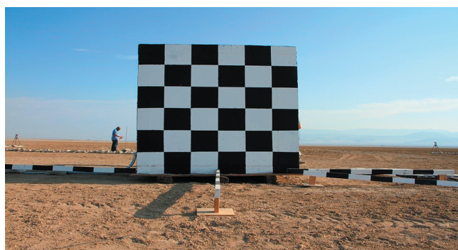
Figure 19 Kasun structure used in HD1.3 M1 propellant testing.
