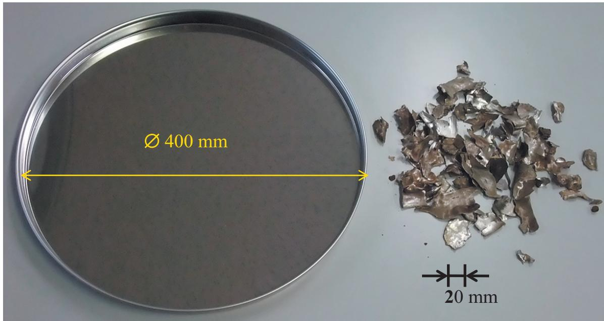
Figure 3 Stainless steel pan before and after explosion in Exp. 3
