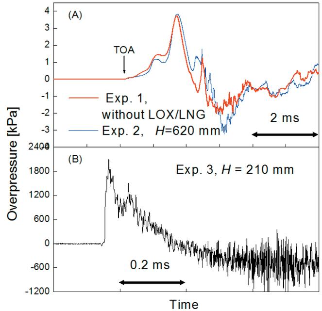
**Figure 2** Time histories of blast wave pressures of Exps. 1 and 2 (A) and Exp. 3 (B)
