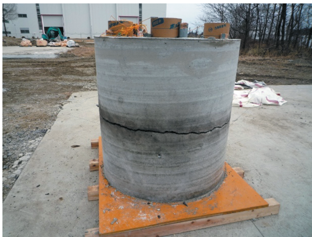
Figure 10 Controlled horizontal fracture along the specified location of the specimen in Exp. No.1.
