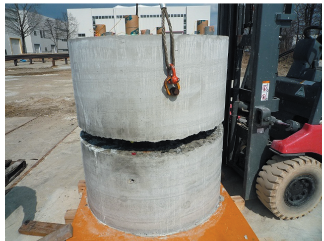
Figure 12 Lifting up of the upper side of the specimen in Exp. No.3.
