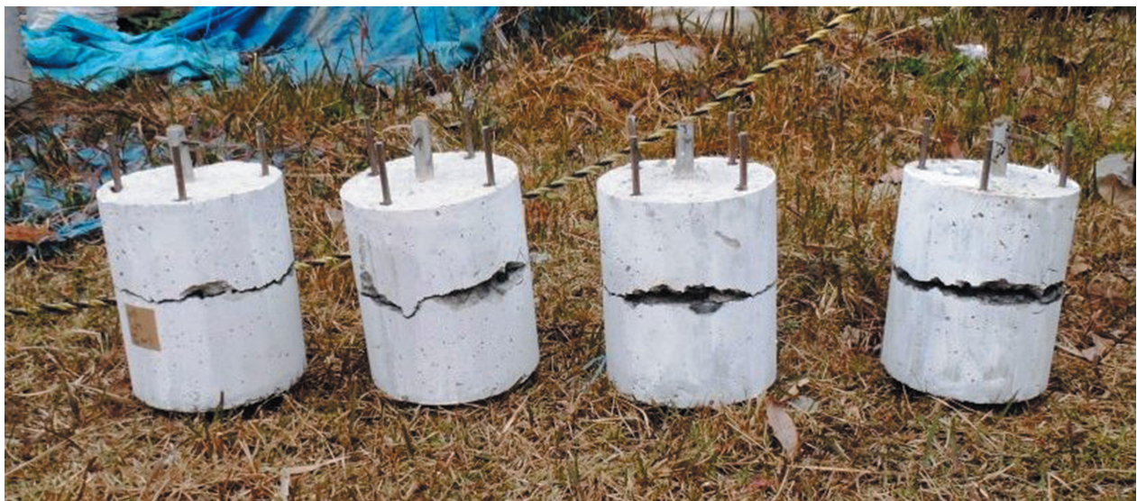
Figure 6 Crack patterns in the model specimen, \phi 200 \times 250 mm after dynamic fracture experiments using CCR as a charge.
