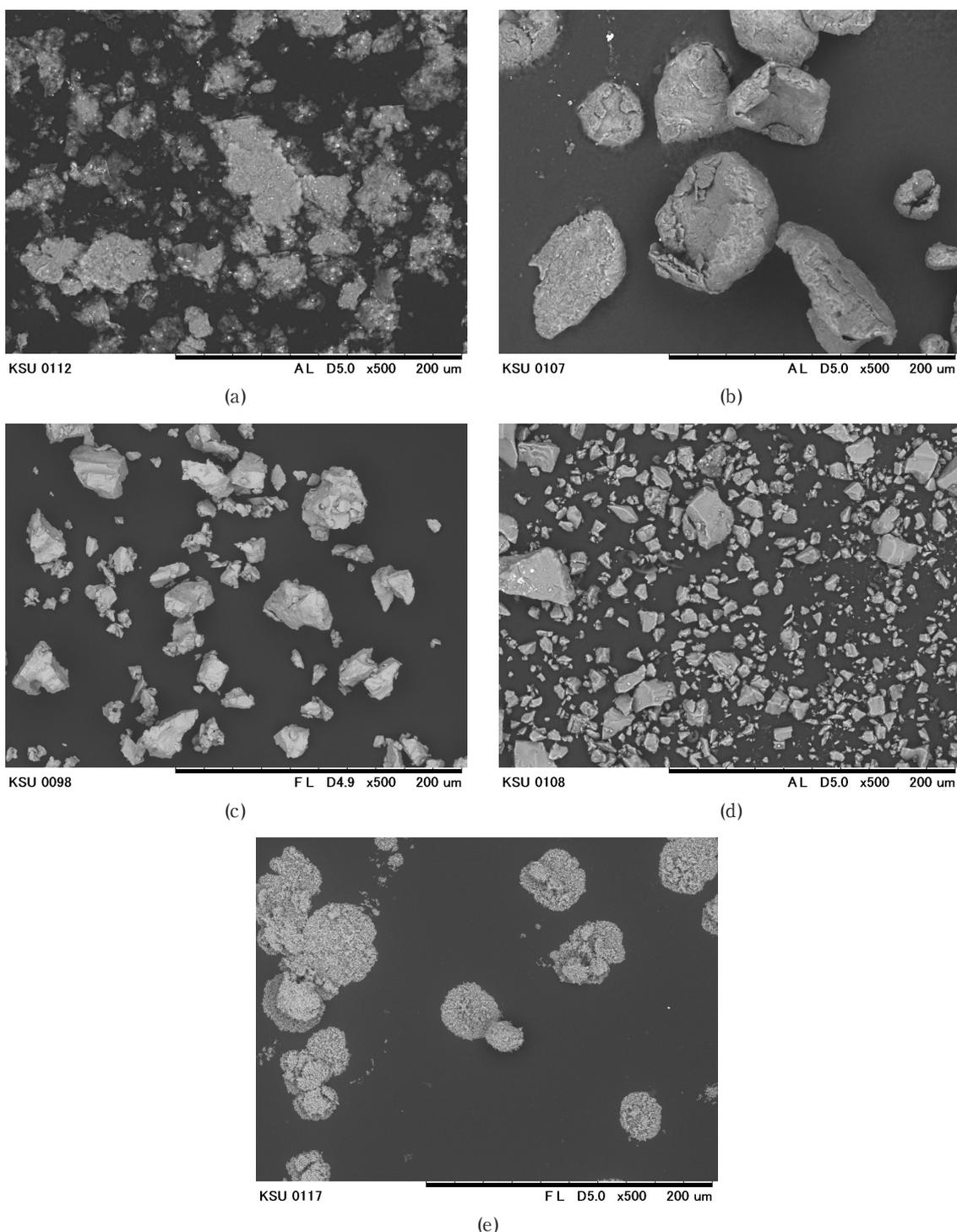
Figure 1 SEM images of (a) Al, (b) Mg, (c) Ti, (d) MgAl and (e)  $\text{Fe}_2\text{O}_3$  used in this study.
