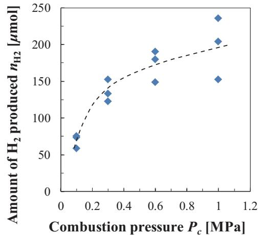
**Figure 6** The relation between  $n_{H_2}$  and  $P_c$ .
