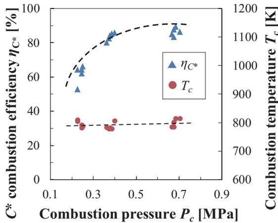
Figure 9 The relation between  $\eta_{C^*}$  and  $T_c$ .
