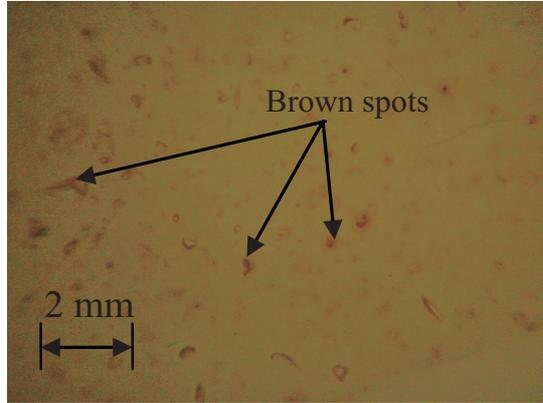
**Figure 4** Carbonaceous residues.
