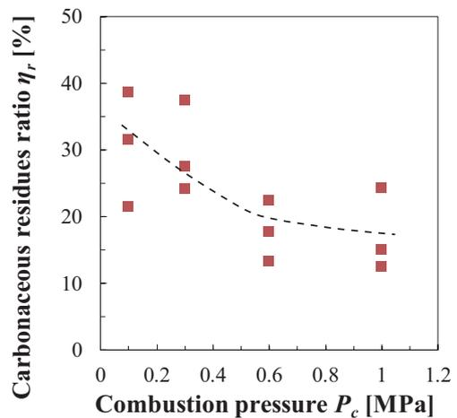
**Figure 7** The relation between  $\eta_r$  and  $P_c$ .
