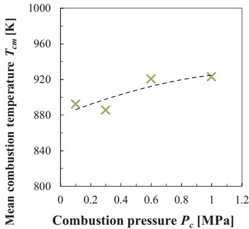
Figure 8 The relation between  $T_{cm}$  and  $P_c$ .
