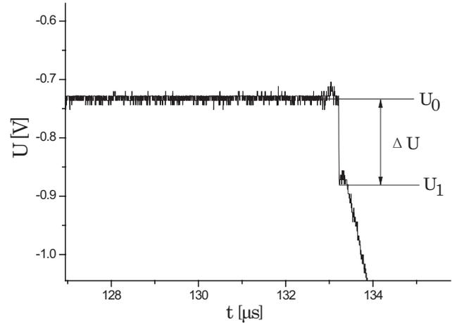
**Figure 4** Typical testing signal of micro manganin piezoresistive sensor.
