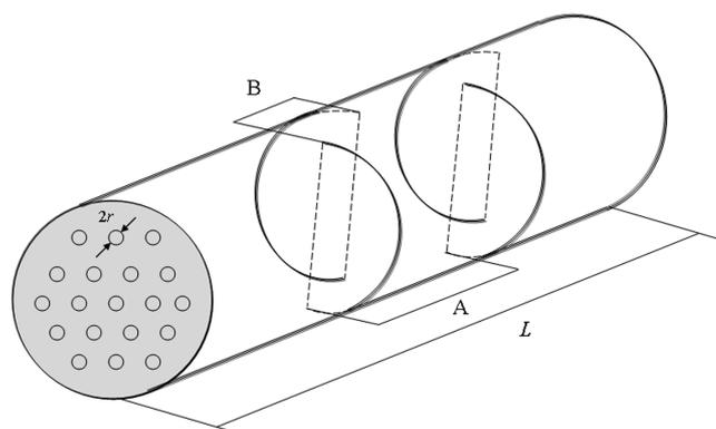
**Figure 1** Schematic of venting method of 19-perforated stick propellants.
