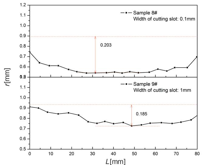
**Figure 6** Variation of internal radius of recovered stick propellant along the length: at different widths of cutting slot.
