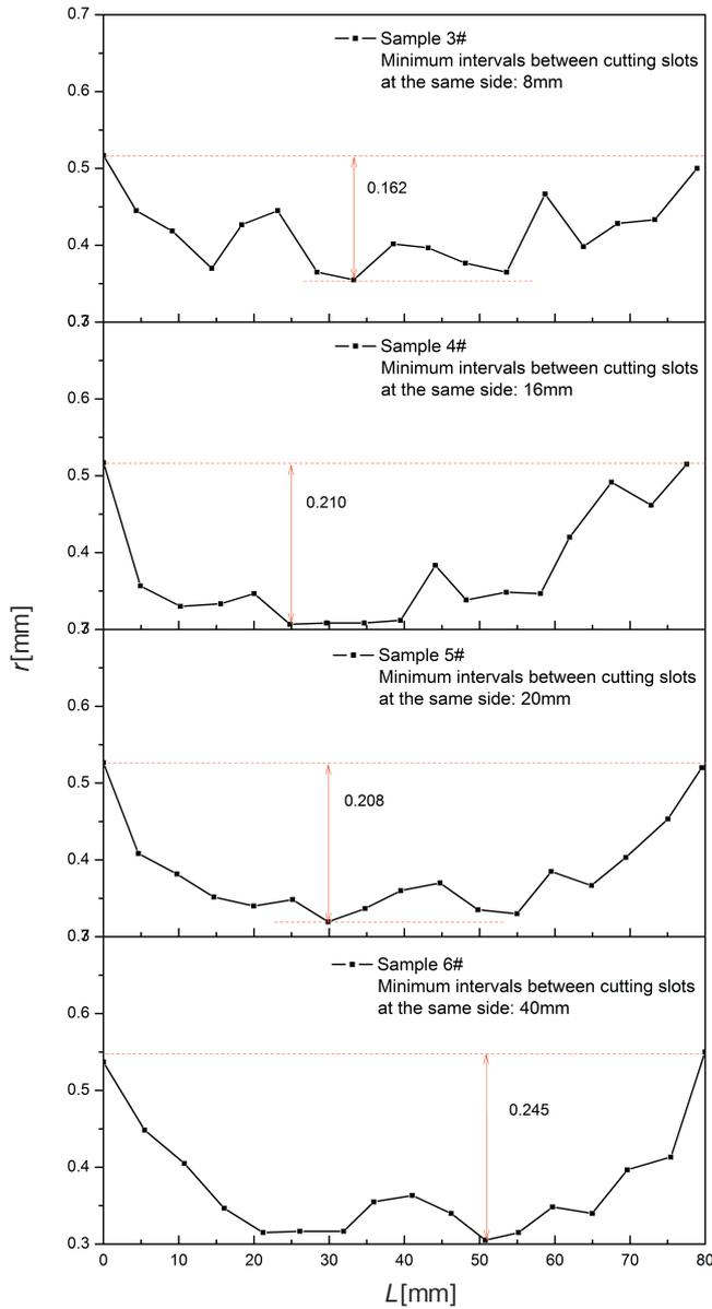
**Figure 4** Variation of internal radius of recovered stick propellant along the length with different intervals between cutting slots at the same side.
