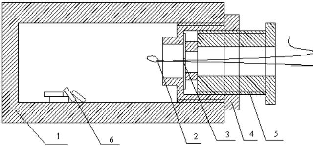
**Figure 2** Schematic of interrupted burning experimental setup: 1-main body, 2-igniter, 3-burst disk, 4, 5-stopper composed of two bolts, 6-propellant.
