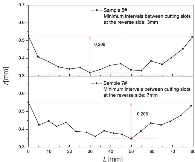
**Figure 5** Variation of internal radius of recovered stick propellant along the length at different minimum intervals between cutting slots at the reverse side.
