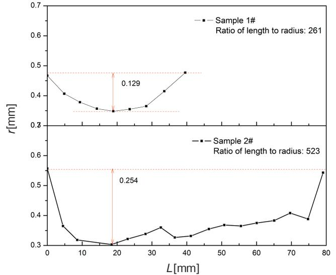
**Figure 3** Variation of internal radius along the length of stick propellant with two kinds of ratios of length to perforation radius: (a) Sample 1#, the ratio of length to perforation radius is 261; (b) Sample 2#, the ratio of length to perforation radius is 523.
