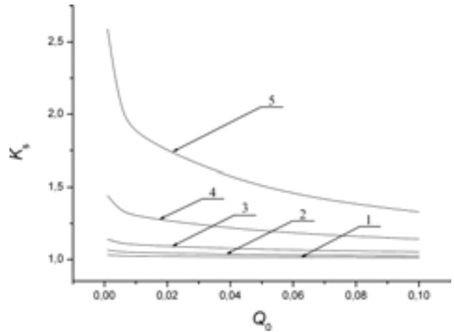
**Fig. 5** Dependence of the safety coefficient  $K_s$  to the lower flammability limit of methane on  $Q_0$  for the error of a determination of LFL  $\sigma_s = 0.05$  (1), 0.1 (2), 0.2 (3), 0.5 (4), 1.0 (5) % (vol).
