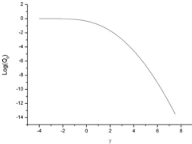
Fig. 2 Dependence of the probability of non fulfillment of the safety conditions (2) on the  $\gamma$  parameter.
