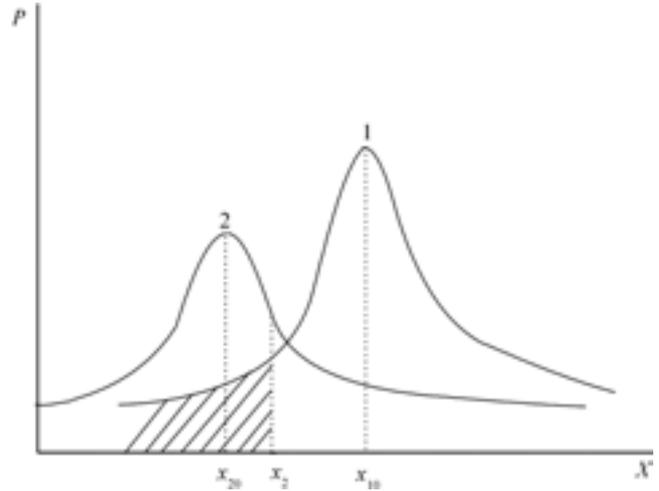
Fig. 1 Qualitative interpretation of safety conditions. 1, 2 – graphs of the functions (3) and (4). The area under the curve is shaded, which is numerically equal to the probability of a fulfillment of the safety condition (2) at the given  $x_2$  value.  $P$  is probability densities for the distributions (3) and (4).
