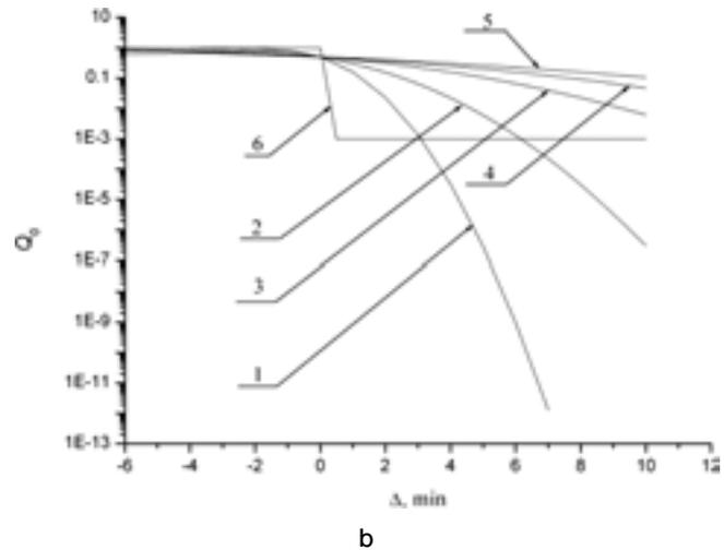
Fig. 3 Dependence of the probability of nonsuccessful evacuation  $Q_0$  on the parameter  $\Delta$  at various  $\sigma_s$ , a -  $\sigma_s = 0.1$  (1), 0.2 (2), 0.4 (3), 1.0 (4) min ; b -  $\sigma_s = 1.0$  (1), 2.0 (2), 4.0 (3), 6.0 (4), 8.0 (5) min. Lines 5 and 6 are the results of the calculations according to the formula (1).
