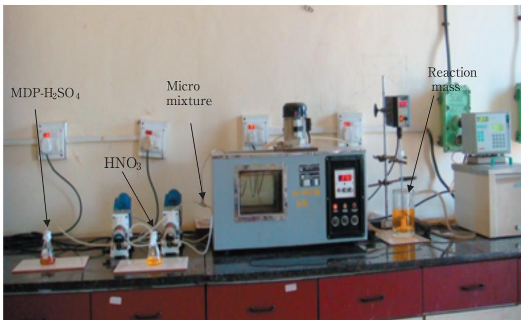
**Fig. 11** Experimental setup for nitration of MDP in micro tubular reactor.
