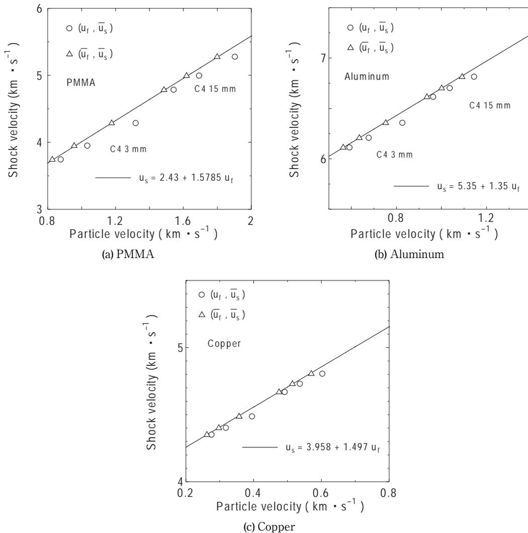
Fig. 2 The relationship between the shock velocity and the particle velocity obtained by numerical simulation.
