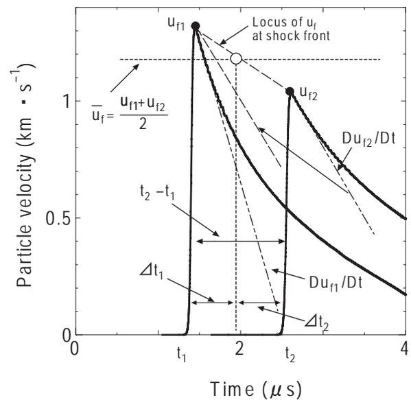
**Fig. 4** Conceptual diagram of our method, Two profiles of particle velocity are drawn using the calculation results in the case of PMMA vs 3 mm C4.
