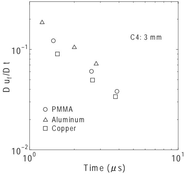
**Fig. 5** The relationship between the arrival times of the shock wave and the slope of the particle velocity.
