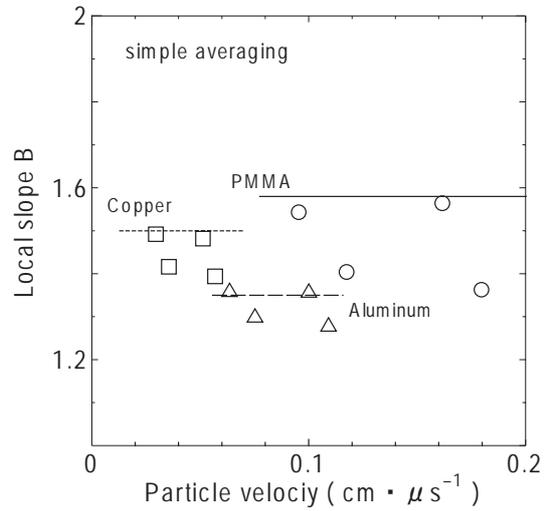
**Fig. 7** The local slope of the Hugoniot obtained by proposed method (simple averaging) The straight lines are an actual slope B.
