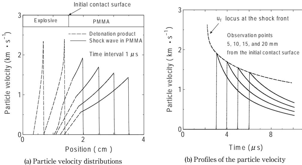
Fig. 1 Typical results of the numerical simulations and the propagation process of decay shock wave in PMMA.
