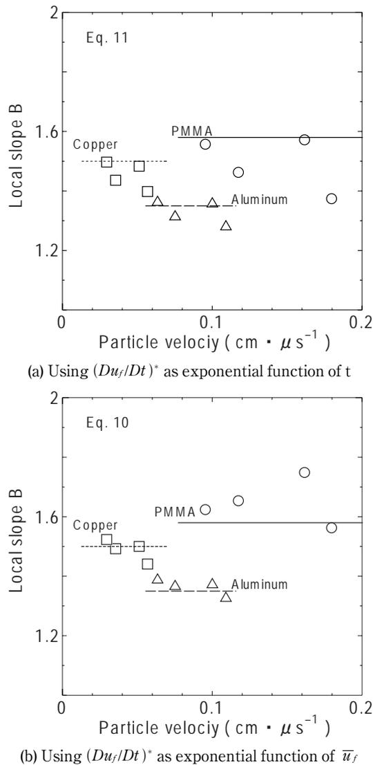
Fig. 8 The local slope of the Hugoniot obtained by proposed method. The straight lines are an actual slope B.
