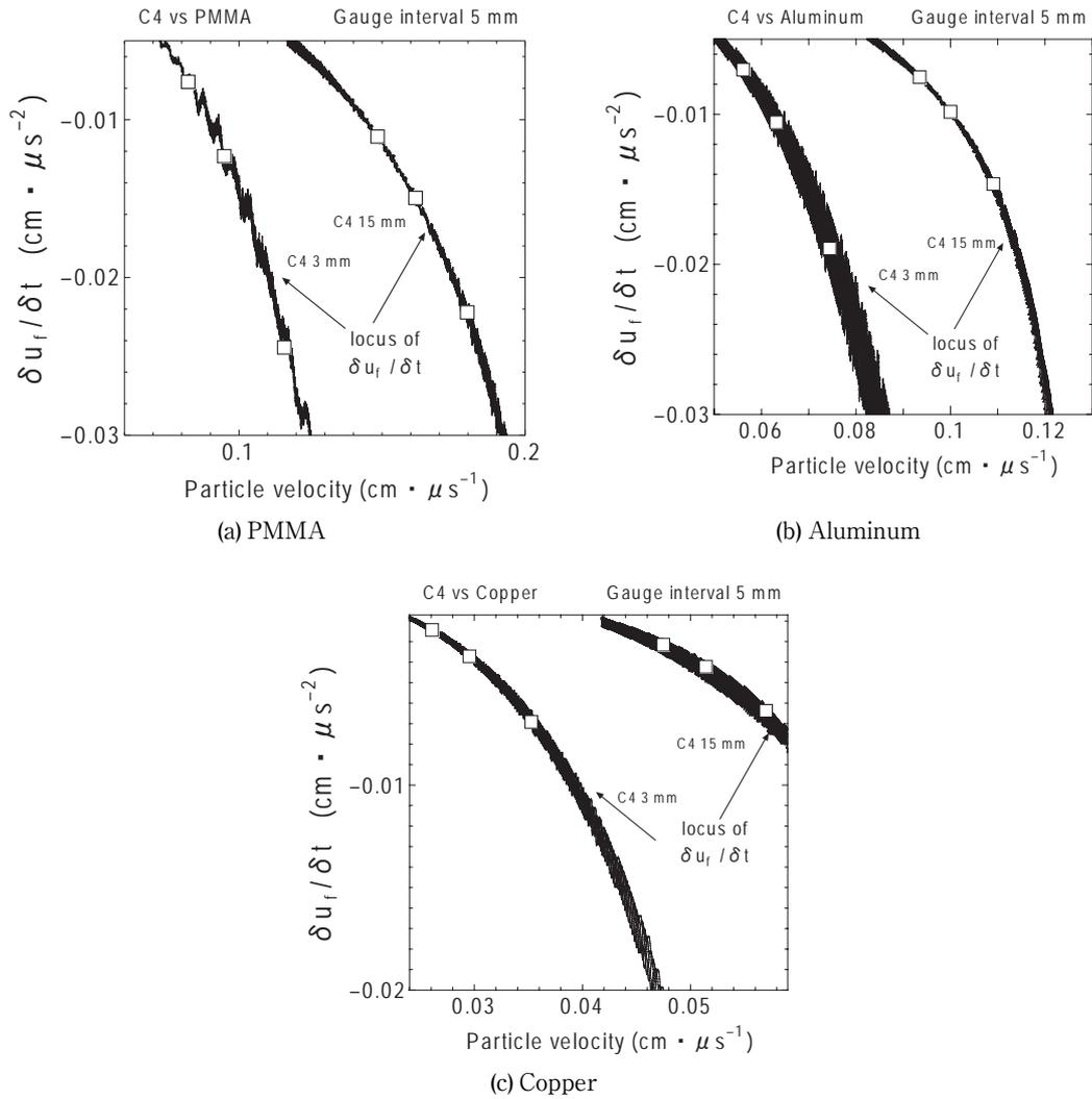
**Fig. 3** The locus of the  $\delta u_f / \delta t$  along the shock front as function of the particle velocity. The symbol  $\square$  corresponds to two points average values of  $\delta u_f / \delta t$  defined by Eq. (7) at  $\bar{u}_f$
