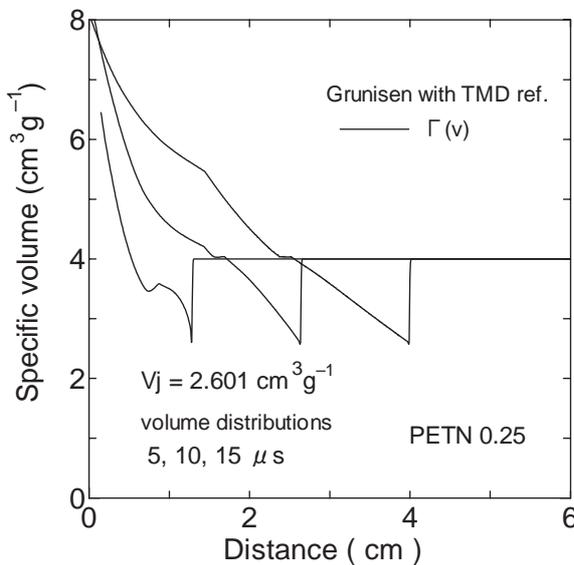
**Fig. 8** The simulation result of the propagation of the detonation wave in PETN. (with specific volume distributions, Initial density ; 0.25 g cm<sup>-3</sup>)
