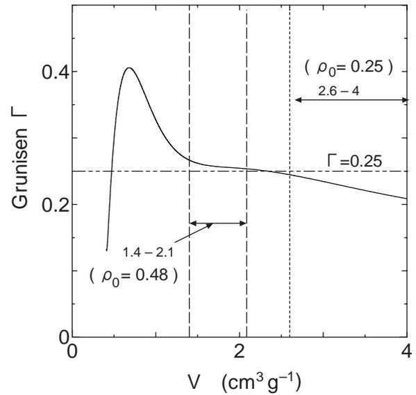
**Fig. 9** Function of Grunisen coefficient for PETN. The regions which have main contribution to calculation results for 0.25 and 0.48 initial density.
