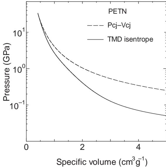
**Fig. 2** The  $p$ - $v$  line along the C-J points, and TMD isentrope for PETN.
