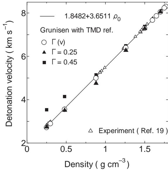
**Fig. 7** The dependence of the detonation velocity of PETN on the initial density, (The sensitivity check of the Grunisen coefficient.)
