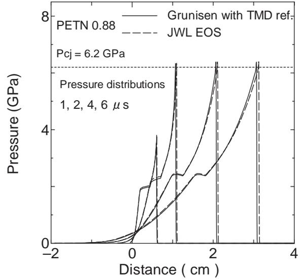
**Fig. 6** The comparison of the simulated detonation wave in PETN. (Initial density ; 0.88 g cm<sup>-3</sup>)
