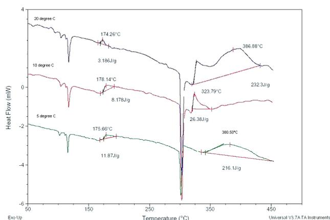
**Fig. 2** DSC plots showing the influence of heating rates on thermal decompositions of a pyrotechnic flash composition (KClO<sub>4</sub>=50 wt.%, Al=23 wt.%, S=27 wt.%)
