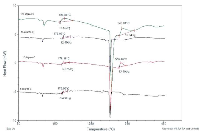
**Fig. 1** DSC plots showing the influence of heating rates on thermal decompositions of a pyrotechnic flash composition (KClO<sub>4</sub>=64 wt.%, Al=23 wt.%, S=13 wt.%)
