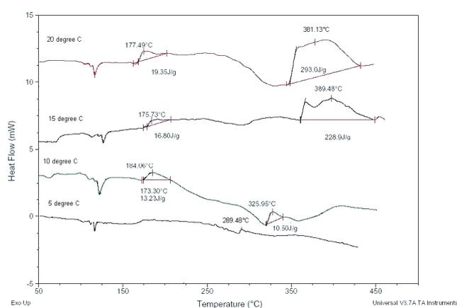
**Fig. 4** DSC plots showing the influence of heating rates on thermal Decompositions of a pyrotechnic flash composition (Ba(NO<sub>3</sub>)<sub>2</sub> =70 wt.%, Al=10 wt.%, S=20 wt.%)
