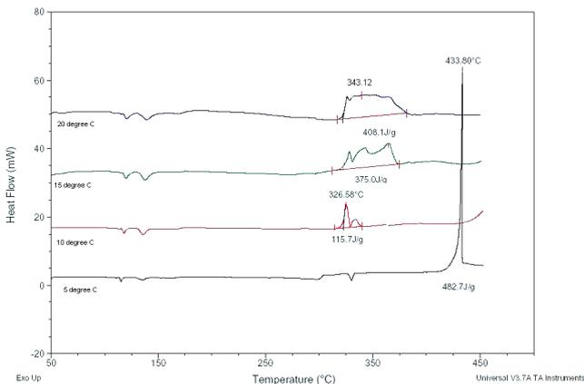
**Fig. 6** DSC plots showing the influence of heating rates on thermal decompositions of a black powder (KNO<sub>3</sub>=50 wt.%, C=25 wt.%, S=25 wt.%)
