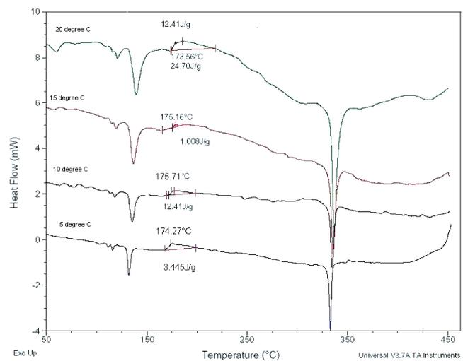
**Fig. 7** DSC plots showing the influence of heating rates on thermal decompositions of a pyrotechnic flash composition (KNO<sub>3</sub>=57wt.%, Mg=32wt.%, S=11wt.%)
