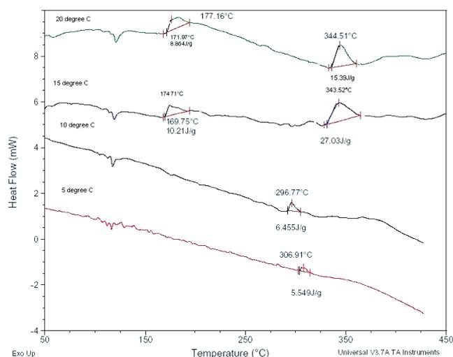
**Fig. 3** DSC plots showing the influence of heating rates on thermal Decompositions of a pyrotechnic flash composition (Ba(NO<sub>3</sub>)<sub>2</sub> =66 wt.%, Al=25 wt.%, S=9wt.%)
