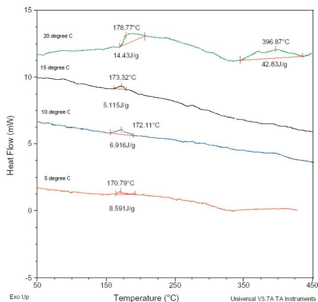
**Fig. 8** DSC plots showing the influence of heating rates on thermal decompositions of a pyrotechnic flash composition (Sr(NO<sub>3</sub>)<sub>2</sub>=30 wt.%, Al=70 wt.%)
