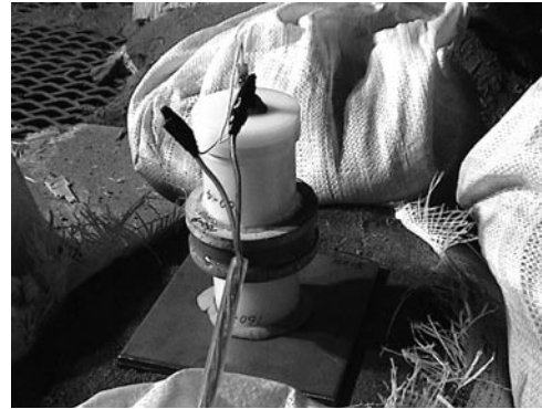
(b) Explosive weight; 160 g, gap length; 35 mm
