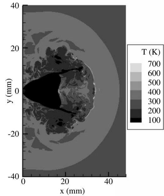
Fig. 9 Temperature contours at 70  $\mu$ s of 70 MPa case.
