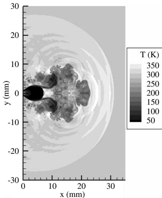
Fig. 2 Temperature contours at 60  $\mu$ s of 10 MPa case.
