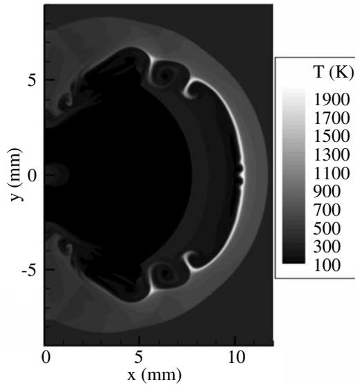
Fig. 8 Temperature contours at 9  $\mu$ s of 70 MPa case.
