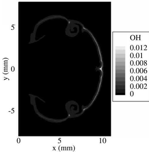
Fig. 4 OH mass fraction contours at 10  $\mu$ s of 40 MPa case.
