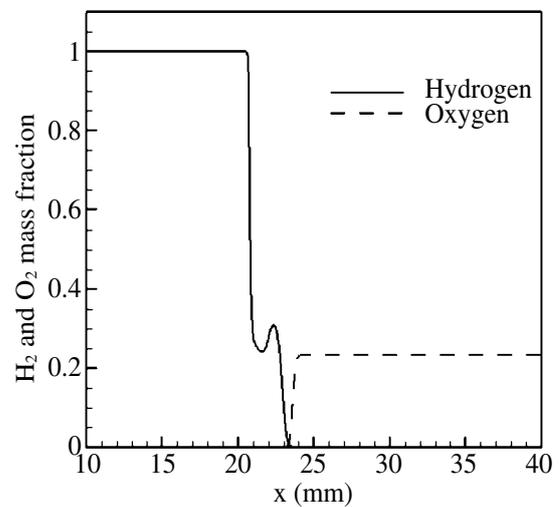
Fig. 7 Hydrogen and oxygen mass fraction contours along the axis at 50  $\mu$ s of 40 MPa case.
