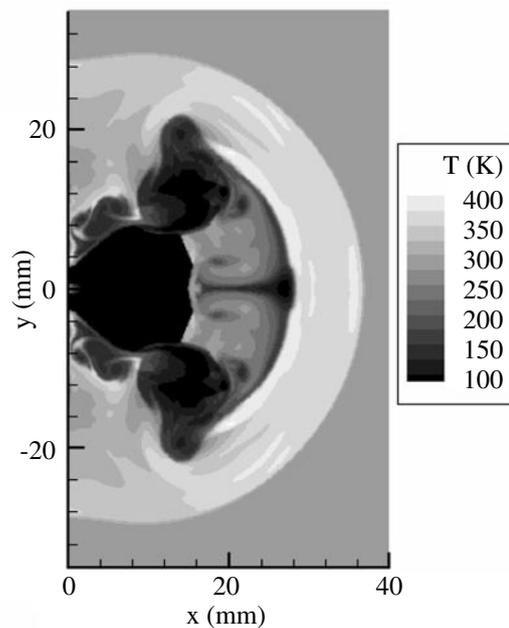
Fig. 11 Temperature contours at 50  $\mu$ s using 100  $\mu$ m grid size of 70 MPa case.
