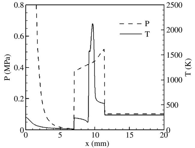
Fig. 5 Pressure and temperature profiles along the axis at 10  $\mu$ s of 40 MPa case.
