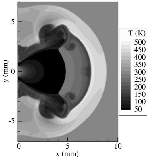
Fig. 1 Temperature contours at 10  $\mu$ s of 10 MPa case.
