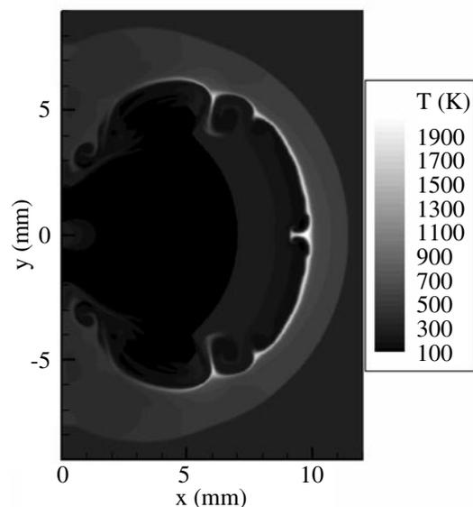
Fig. 3 Temperature contours at 10  $\mu$ s of 40 MPa case.
