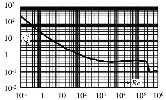
Fig. 3 Plot of  $C_D$  vs.  $Re^5$ .
