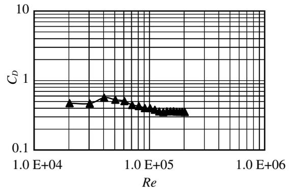
Fig. 4  $C_D$  of a No. 5 sphere shell by wind tunnel.
