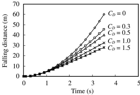
Fig. 2 Plot of calculated falling distance vs. time for No. 2 shell.
