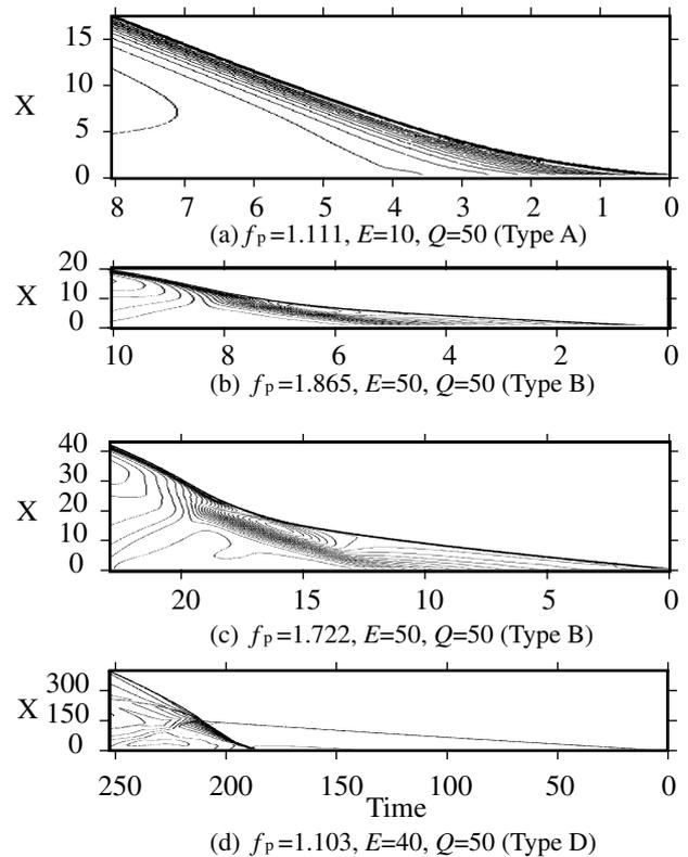
**Fig. 2** T-x diagrams of density distributions of the one-dimensional piston-supported detonations.  $f_p$ ; degree of overdrive,  $E$ ; activation energy,  $Q$ ; heat release.
