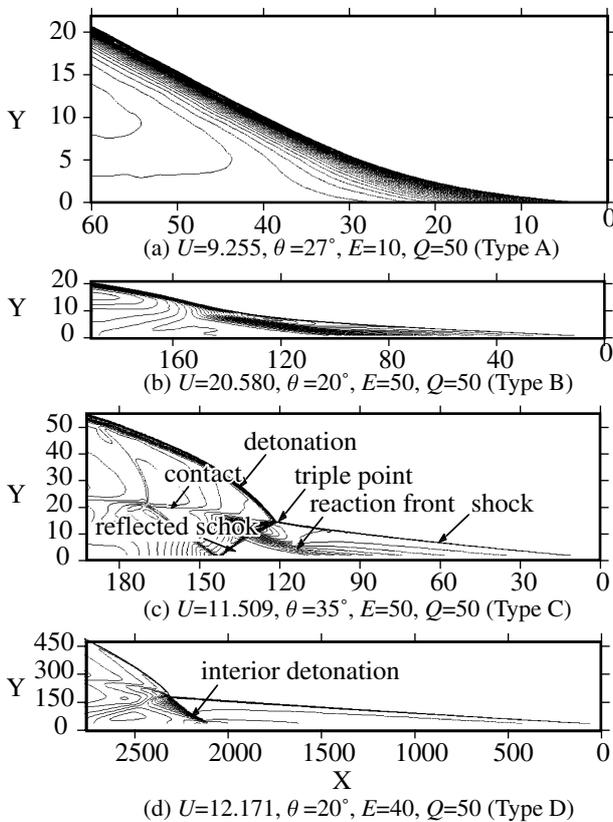
**Fig. 1** The density distributions of the wedge-induced detonations.  $U$ ; incoming flow speed,  $\theta$ ; wedge angle,  $E$ ; activation energy,  $Q$ ; heat release.
