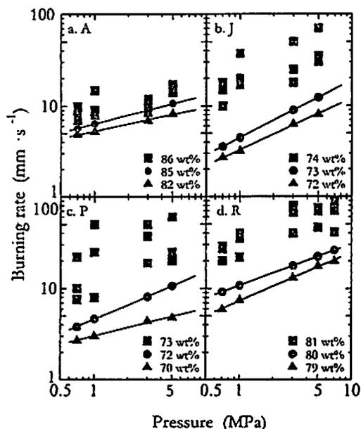
Fig.2 Burning rate characteristics of propellants A, J, P, and R
