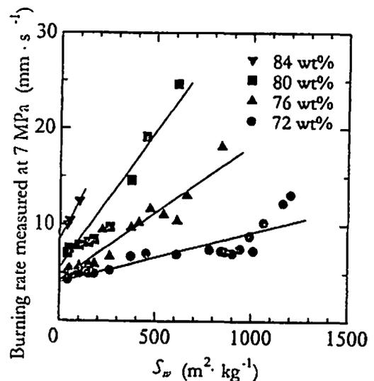
Fig.5 Relationship between burning rate at 7 MPa and  $S_w$
