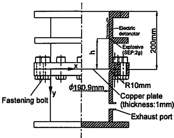
Fig. 1 Schematic diagram of experimental device for the eccentric spherical metal sheet forming.
