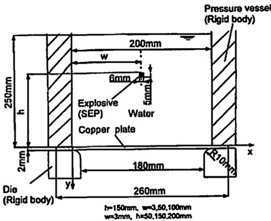
Fig. 7 Simulation model for free metal sheet forming.
