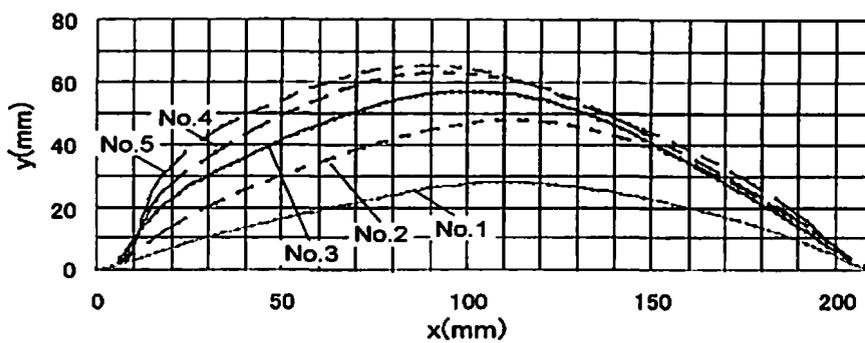
Fig. 3 Measurement results on the surface shape of copper plate.
