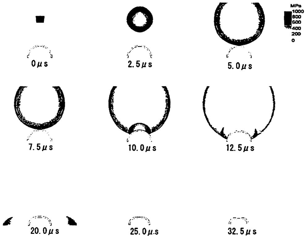
Fig. 11 Pressure contours and deformation process of copper pipe for each times by simulation results.
