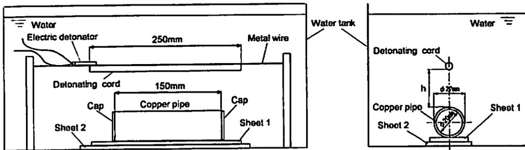
Fig. 5 Schematic diagram of experimental setting for copper pipe forming using underwater shock wave generated by underwater explosion of explosive.
