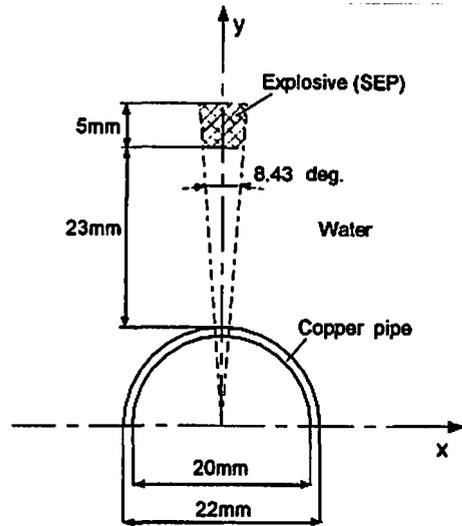
Fig. 8 Simulation model for copper pipe forming using underwater shock wave.
