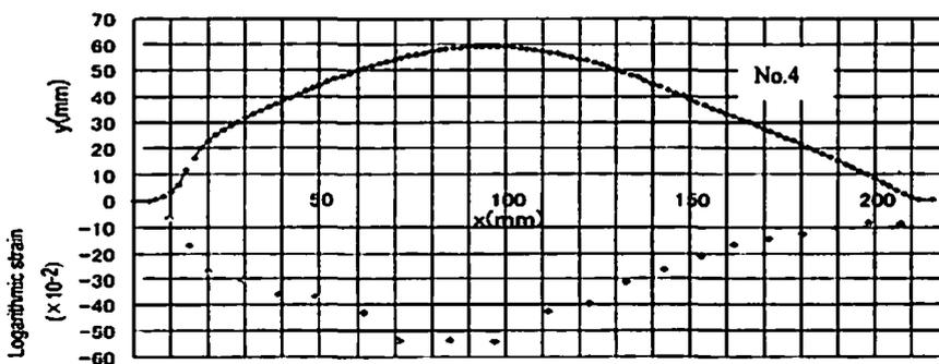
Fig. 4 Distribution of thickness logarithmic strain of copper plate to the measurement results of surface shape of copper plate (No.4).
