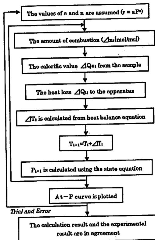
Fig.2 Flow chart of the simulation.
