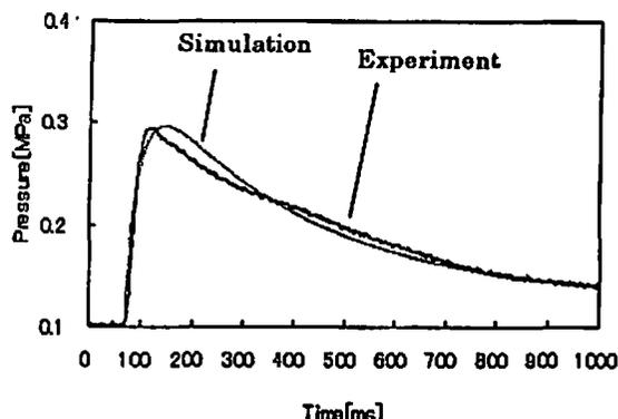
Fig.4 Comparison of the experimental data of ignition charge and the simulation result
