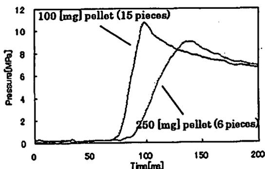
Fig.3 The effect of heat loss to the pressure curve
