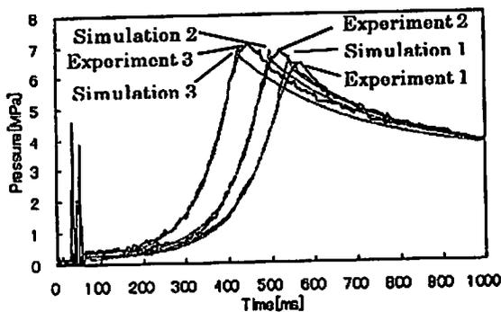
Fig.6 Reproducibility of the pressure curve of single base propellant.
