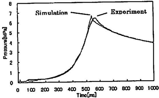
Fig.5 Comparison of the experimental result of single base propellant and the simulation result (1 piece)
