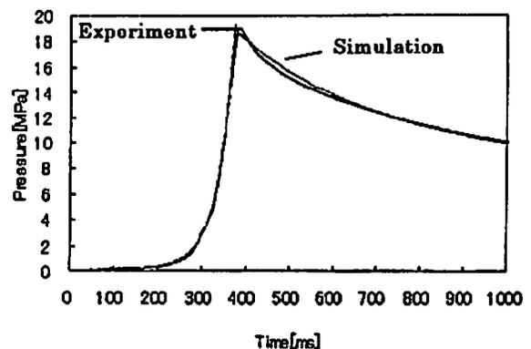
Fig.7 Comparison of the experimental data of single base propellant and the simulation result (2 pieces)
