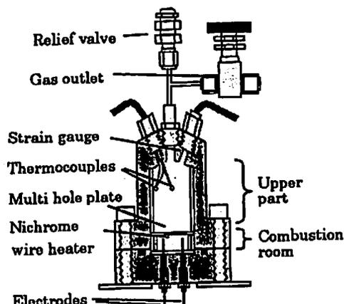
Fig. 1 52ml deflagration test apparatus.
