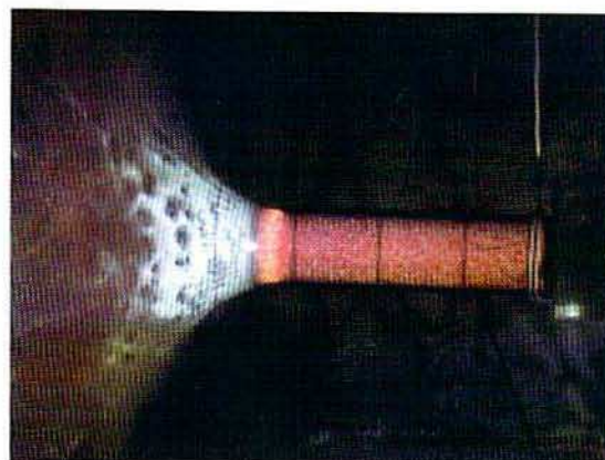
Fig.2 High-speed photographs of detonation behavior of ANFO with the PVC tube.
