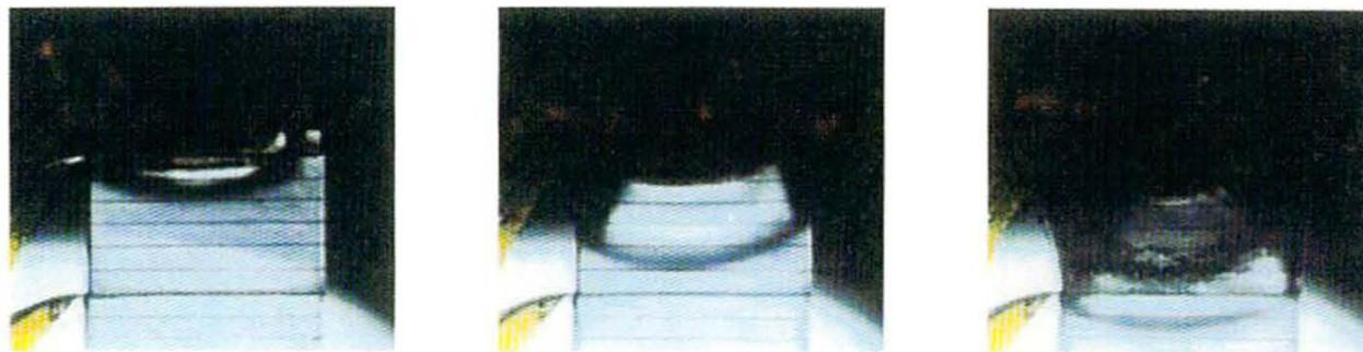
Fig. 7 High-speed camera photographs of shock wave propagation in PMMA gap
