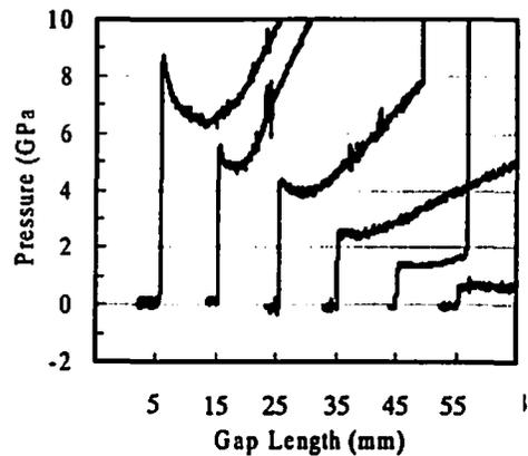
Fig. 2 Pressure profiles of shock waves in PMMA gap measured by manganin gauges
