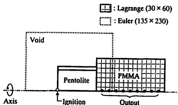
Fig. 3 Configuration of the analysis model of shock propagation
