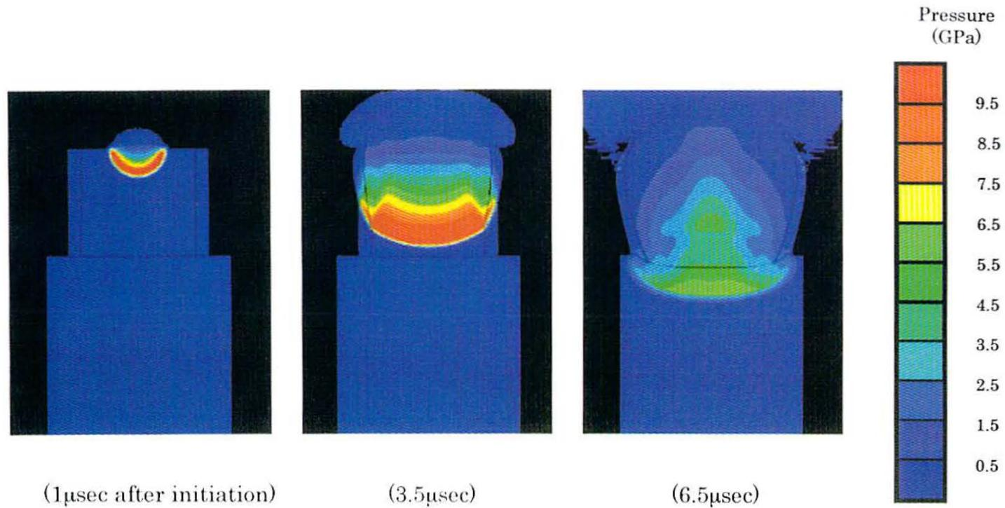
Fig. 6 Pressure contours of shock propagation through PMMA gap calculated with AUTODYN<sup>®</sup>-2D
