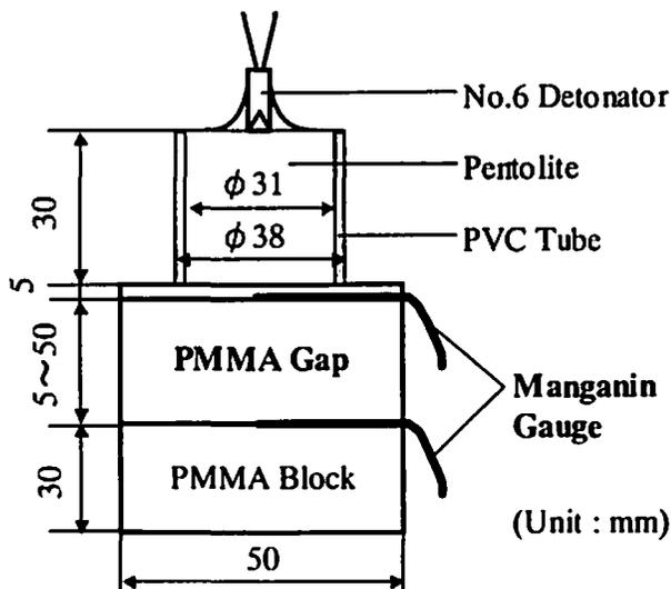
Fig. 1 Experimental arrangement of shock attenuation in PMMA
