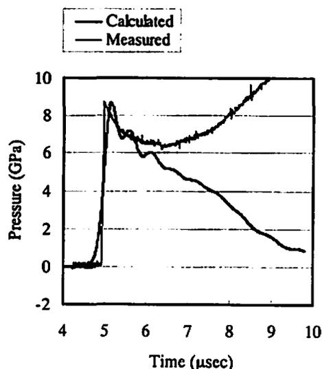
Fig. 4 Comparison of measured and calculated shock pressure profiles
