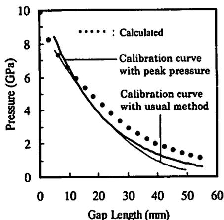
Fig. 5 Shock attenuation in PMMA computed by AUTODYN®-2D compared with experimental results
