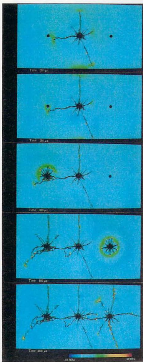
Fig. 9 Distribution of maximum principal stress and crack propagation process for the case of conventional DS detonator initiation
