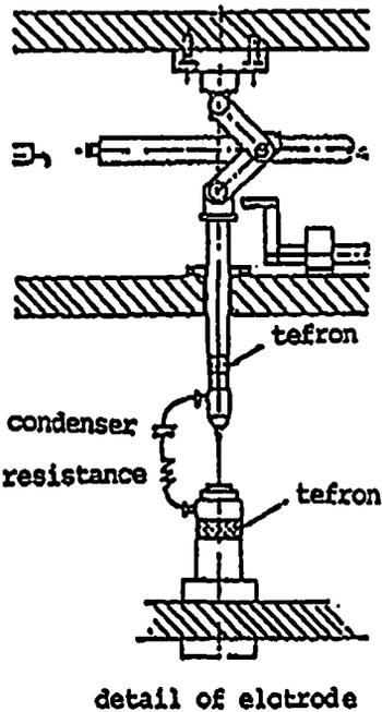
Fig. 1 Approaching electrode apparatus
