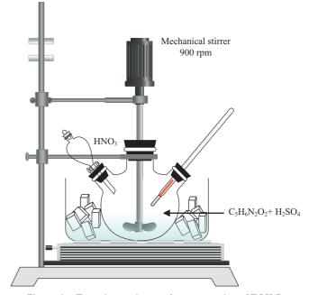
Figure 4 Experimental setup for preparation of FOX-7.
