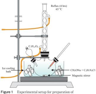
Figure 1 Experimental setup for preparation of 2-methylpyrimidine-4,6-diol.
