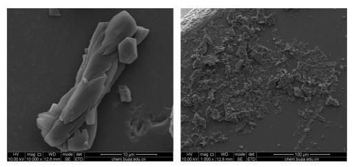
Figure13 SEM photos of FOX-7 crystals.
