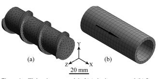
Figure 1 Finite element model of (a) single screw and (b) flow channel.
