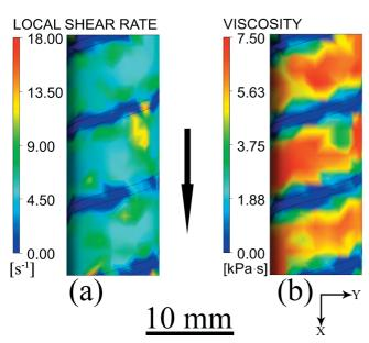
Figure 3 (a) Shear rate and viscosity (b) distributions in the surface of the fluid.  $(T = 50 \text{ °C}, r = 10 \text{ rmin}^{-1}, c = 1.20 \text{ mL} \cdot \text{g}^{-1})$
