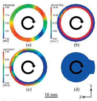
Figure 2 (a) Pressure, (b) velocity, (c) viscosity, and (d) screw distributions in YZ section.  $(T = 50 \text{ °C}, r = 10 \text{ r}\cdot\text{min}^{-1}, c = 1.20 \text{ mL}\cdot\text{g}^{-1})$
