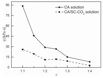
Figure 11 The average viscosity with different solvent content. (T = 50 °C, r = 10 r·min<sup>-1</sup>)
