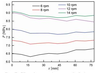
Figure 7 Effects of screw speed on pressure distributions.  $(T = 50 \text{ °C}, c = 1.20 \text{ mL} \cdot \text{g}^{-1})$
