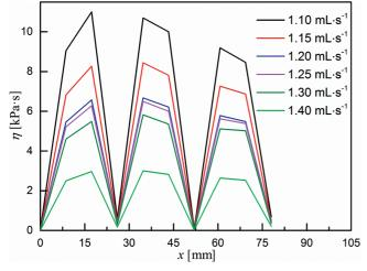
**Figure10** Effects of solvent content on viscosity distributions.  $(T = 50 \text{ }^{\circ}\text{C}, r = 10 \text{ r} \text{min}^{-1})$
