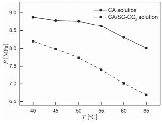
**Figure 9** The average pressure at various temperatures.  $(r = 10 \text{ rmin}^{-1}, c = 1.20 \text{ mL} \cdot \text{g}^{-1})$
