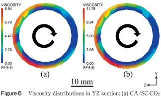
Figure 6 Viscosity distributions in YZ section: (a) CA/SC-CO<sub>2</sub> solution, (b) CA solution.  $(T = 45 \text{ °C}, r = 10 \text{ r·min}^{-1}, c = 1.20 \text{ mL} \cdot \text{g}^{-1})$
