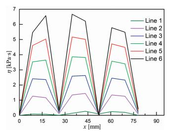
Figure 4 Viscosity distributions along the lines in XZ section.  $(T = 50 \text{ °C}, r = 10 \text{ r} \cdot \text{min}^{-1}, c = 1.20 \text{ mL} \cdot \text{g}^{-1})$
