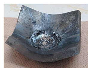
Figure 4 Conditions of witness plate after the test. (Positive result : left, Negative result : right)
