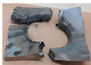
Figure 4 Conditions of witness plate after the test. (Positive result : left, Negative result : right)
