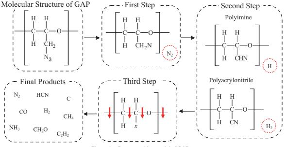
Figure 1 Decomposition model of GAP.
