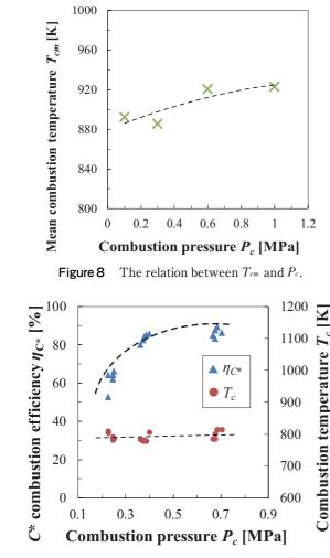
**Figure 9** The relation between  $\eta_{C^*}$  and  $T_c$ .
