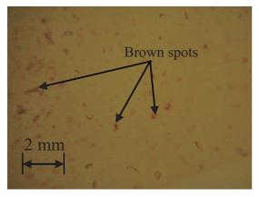
Figure 4 Carbonaceous residues.
