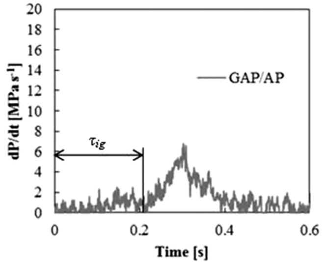
**Figure 7** Temporal differentiations of the pressure in the secondary combustor.
