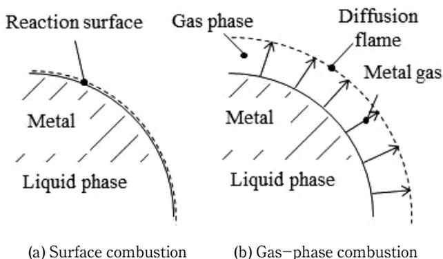
Figure 2 Combustion types of metal particles.
