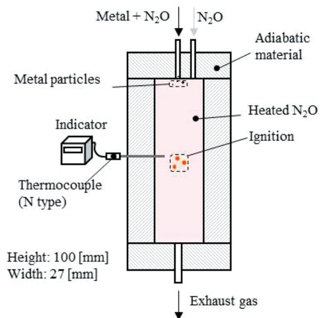
Figure 3 Electric furnace.
