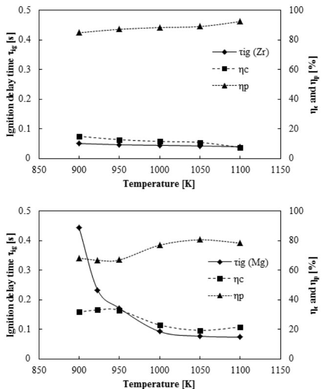
**Figure 5** Relation between the electric furnace temperature and ignition delay time or the ratio of  $\tau_c$  to  $\tau_p$  to the ignition delay time at 0.1 MPa: (a) zirconium 45 μm and (b) magnesium 45 μm.
