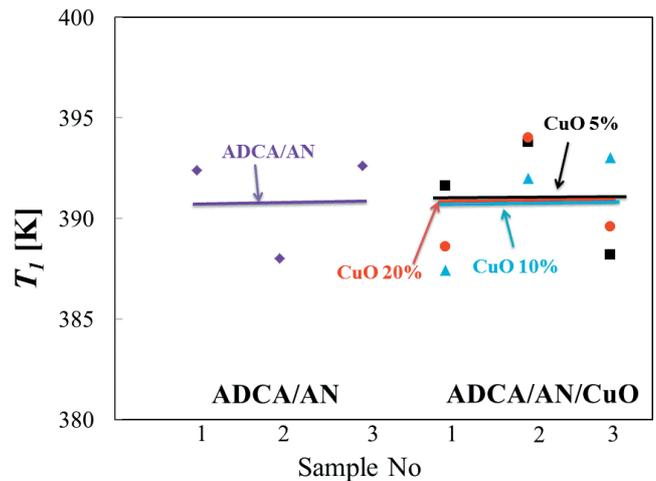
**Figure 5** Onset temperature of the condensed phase for ADCA/AN based mixtures.
