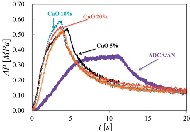
**Figure 3** Pressure-time history of ADCA/AN based mixtures from rate-of-pressure-rise test.
