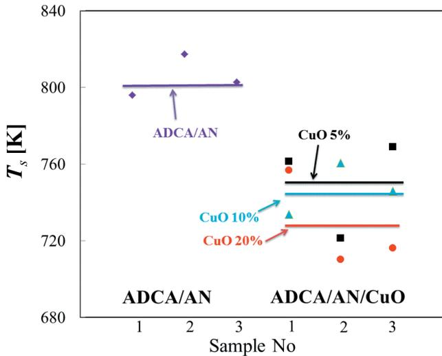
**Figure 6** Burning surface temperature for ADCA/AN based mixtures.
