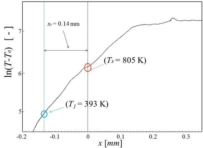
**Figure 4** An example of  $\ln(T-T_0)$  vs  $x$  curve for ADCA/AN mixture at 2 MPa.
