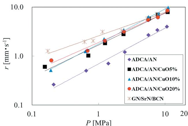
Figure 2 Linear burning rates for ADCA/AN based mixtures.
