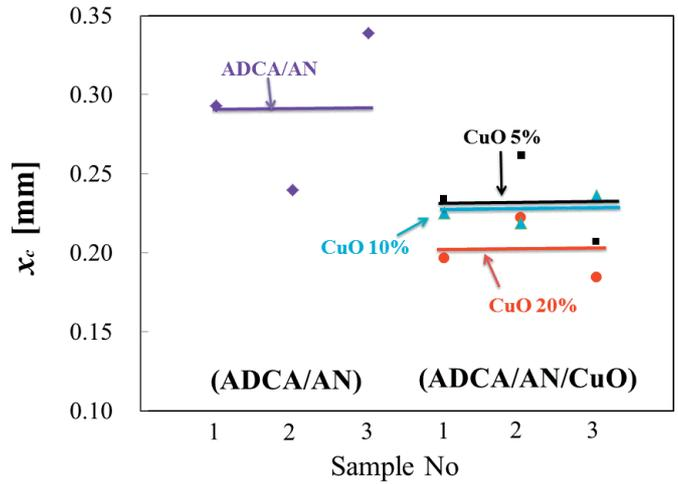
**Figure 7** Thickness of condensed phase for ADCA/AN based mixtures.
