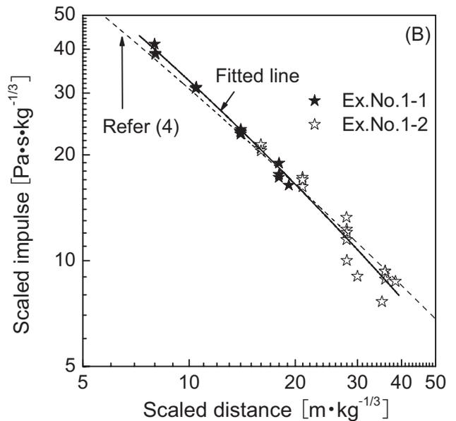
Figure 4 Peak overpressure (A) and scaled impulse (B) of Ex. No. 1 for surface burst with respect to scaled distance.
