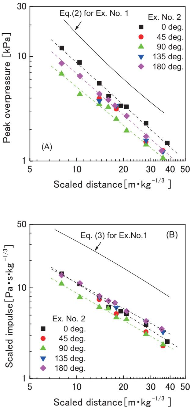
Figure 5 Peak overpressure (A) and scaled impulse (B) for ECM of Ex. No. 2 with respect to scaled distance.
