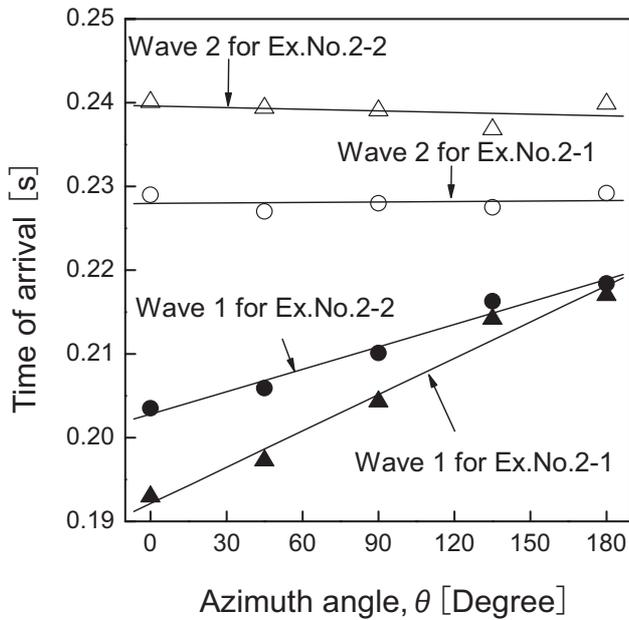
Figure 6 Time of arrival of Wave 1 and Wave 2 at 76 m for Ex. No. 2-1 and 2-2.
