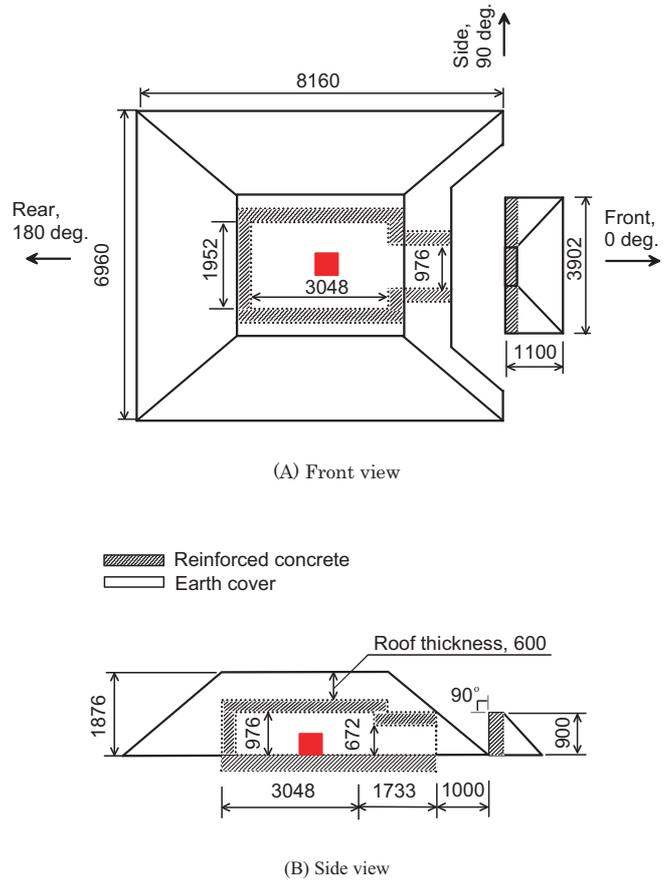
Figure 1 Model of ECM with barricade used in 160 kg test (Unit: mm).
