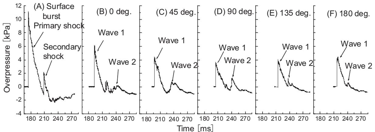
Figure 3 Time histories of blast wave pressure at 76 m for Ex. No. 1-1(A) and for Ex. No. 2-1(B, C, D, E, F).
