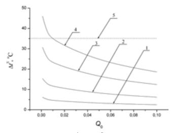
Fig. 4 Dependence of  $\Delta t^s$  on  $Q_0$  for the error of a determination of the flash point  $\sigma_s=2(1)$ , 5(2), 10 (3), 15 (4)°C. Line5is the graph of the dependence (11).
