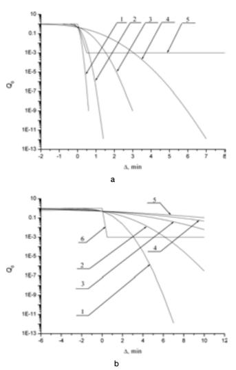
**Fig.3** Dependence of the probability of nonsuccessful evacuation  $Q_0$  on the parameter  $\Delta$  at various  $\sigma_s$ .  $a - \sigma_s = 0.1$  (1), 0.2 (2), 0.4 (3), 1.0 (4) min ;  $b - \sigma_s = 1.0$  (1), 2.0 (2), 4.0 (3), 6.0 (4), 8.0 (5) min. Lines 5 and 6 are the results of the calculations according to the formula (1).
