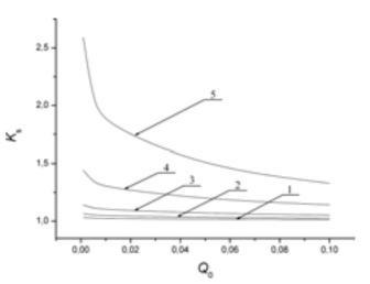
**Fig. 5** Dependence of the safety coefficient  $K_s$  to the lower flammability limit of methane on  $Q_0$  for the error of a determination of LFL  $\sigma_s = 0.05$  (1), 0.1 (2), 0.2 (3), 0.5 (4), 1.0 (5) % (vol.).
