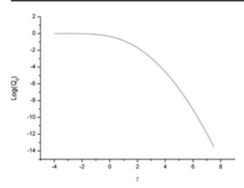
**Fig.2** Dependence of the probability of non fulfillment of the safety conditions (2) on the  $\gamma$  parameter.
