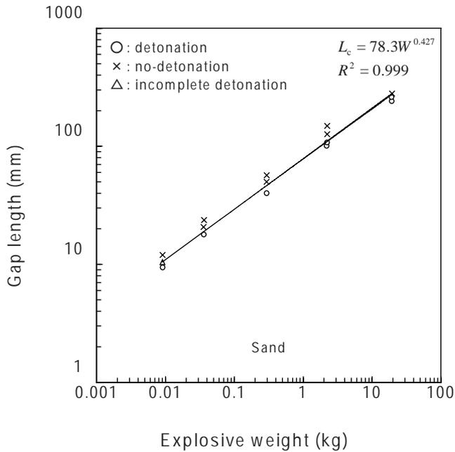
Fig. 4 Relation of explosive weight and gap length for sand.
