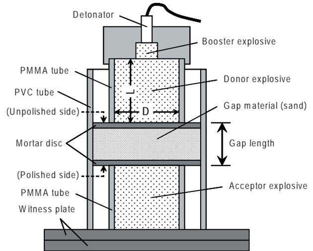
Fig. 1 (b) Experimental setup for sand gap (explosive weight up to 2.5 kg).
