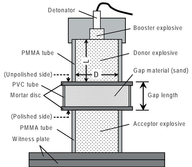
Fig. 1 (c) Experimental setup for sand gap (explosive weight of 20 kg).
