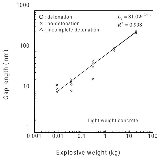
**Fig. 3** Relation of explosive weight and gap length for light weight concrete.
