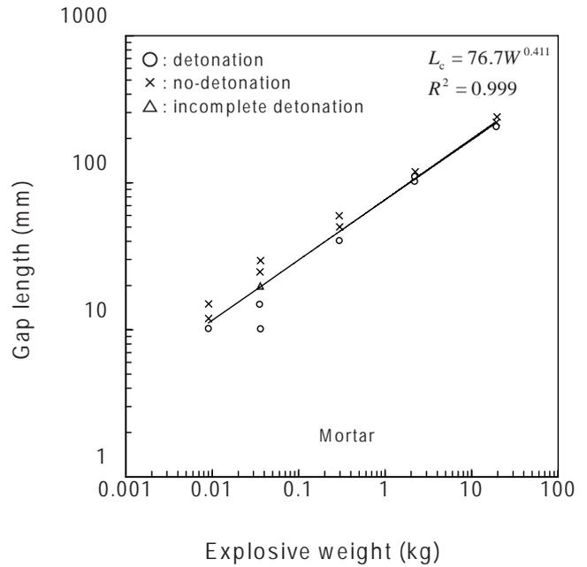
**Fig. 2** Relation of explosive weight and gap length for mortar.
