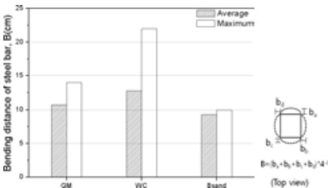
Fig. 6 Bending of reinforced beam by stemming material.
