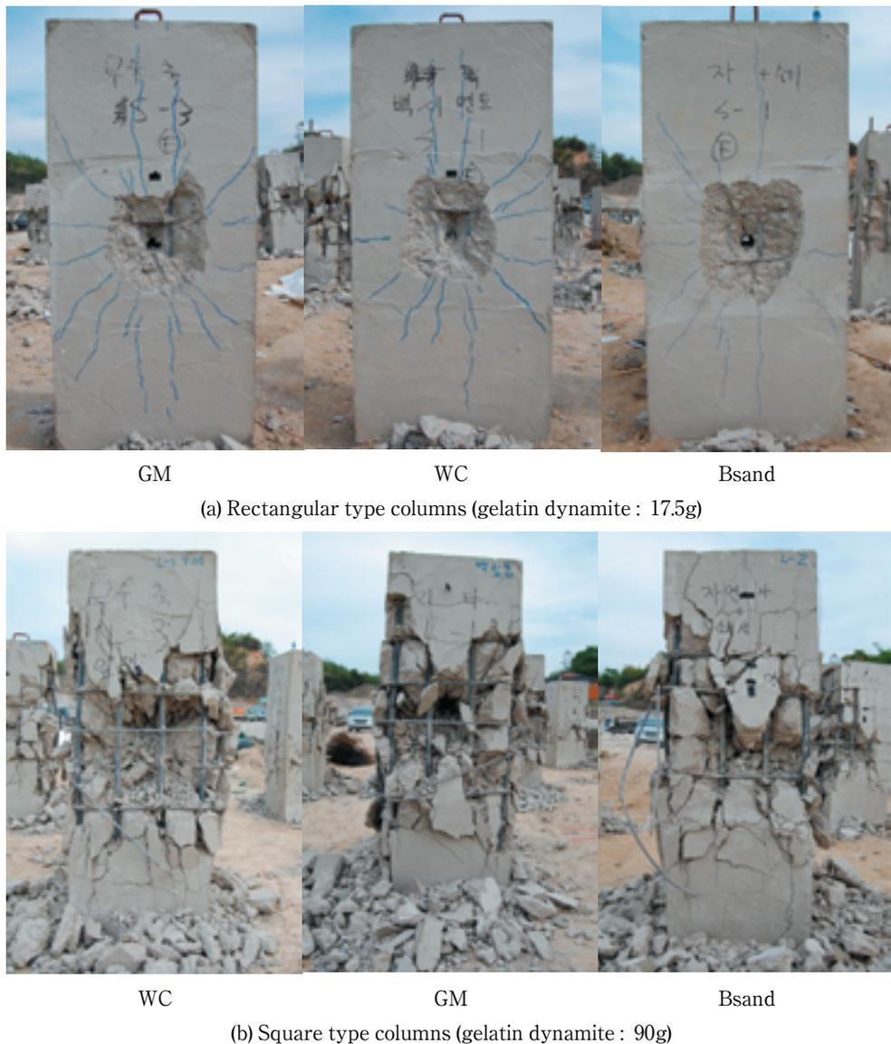
**Fig. 4** Fracture pattern in a single hole blast columns (Front view).
