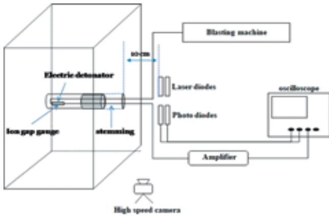
Fig. 3 Schematic description for full scaled-column blast and dynamic data measurements.
