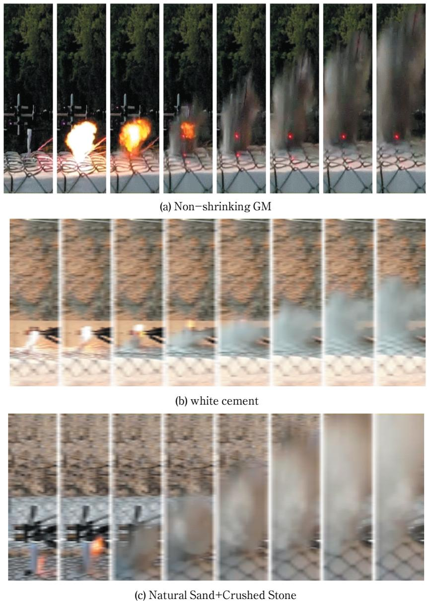
Fig. 9 High speed camera images of flying stemming materials (1200 frames/sec).
