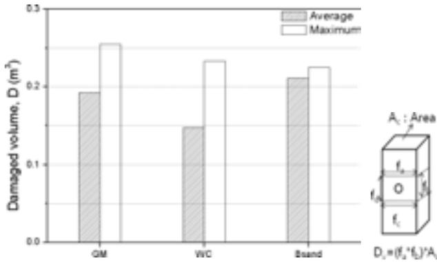
(b) Damaged volume of square type column specimen
