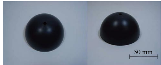
Fig. 2 Shell case made by biodegradable plastic.
