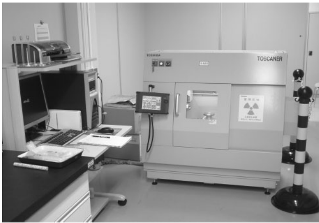
Fig. 1 High resolution micro X-ray computed tomography (CT) system (TOSCNAR 30900 \mu hd, Toshiba co.).
