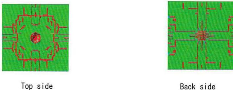
Fig.13 Simulated result of cracking (H-102)
