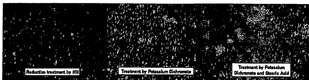
Fig. 8 Microscopic pictures of surface-treated Mn particles (X600)
