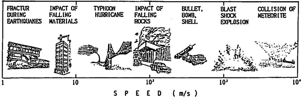
Fig. 1 Approximate speed of various accidents might fall upon structures
