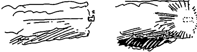
Two consecutive frames from cut K7 in the Kråkemåla quarry Fig. 2 Charge detonating part-way in the air. Sketch after high speed filming frames.
