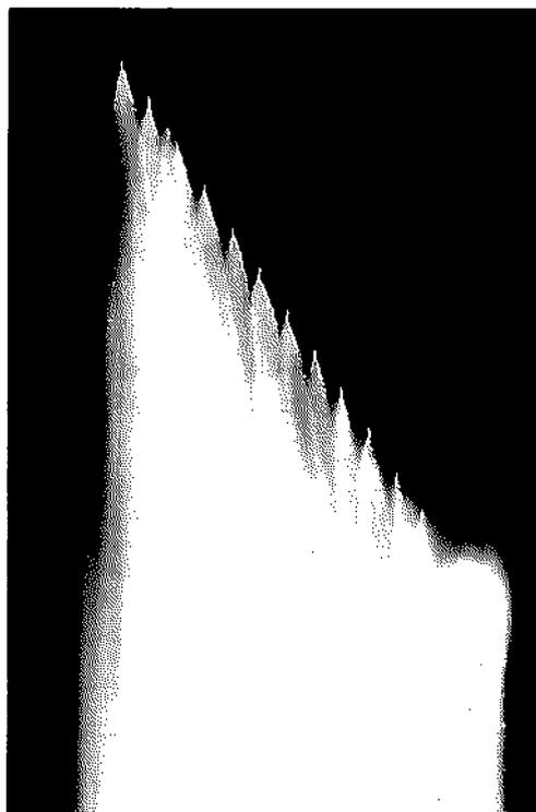
Fig. 2 A streak record of a detonating PBX sample.
