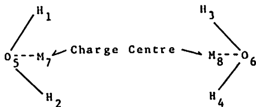
Fig. 1 Definition of distances used in the MCY and the RWK2 Potentials
